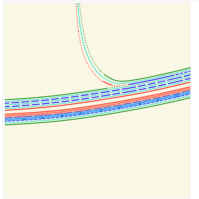
Figure 47: Bad case 3: the GPS data is straightened up over time, but the VA fails at changing the path into the correct one. This is caused by the added lane change transitions being too influential - since there is no lane change, a straight path is enforced. There are also no lane markers to get help from, as the detector again reports 0 confidence.
