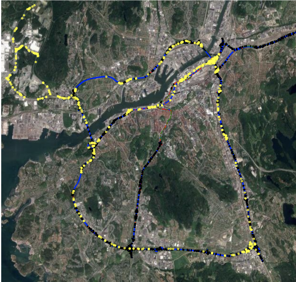
Figure 7: Google map image of Gothenburg, courtesy of Google, Inc., layered with the TomTom map. Blue lines represent roads and lanes. Red, black and yellow markers indicate traffic signs, stop lights, junctions and other road-related objects.
