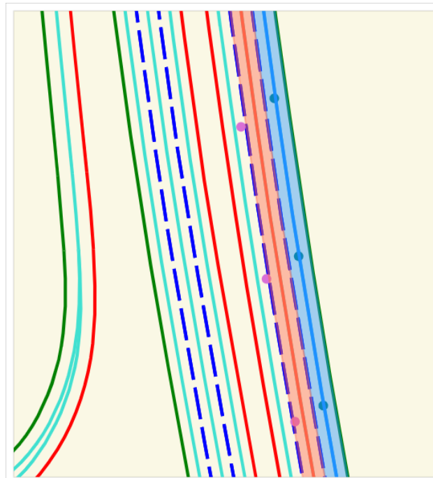
Figure 46: Bad case 2: left and right lane marker types are correctly reported as (dashed, solid), as for the true states, but the GPS error is too big. This leads to the middle lane being identified as the most probable one, even though it has incorrect lane markers.
