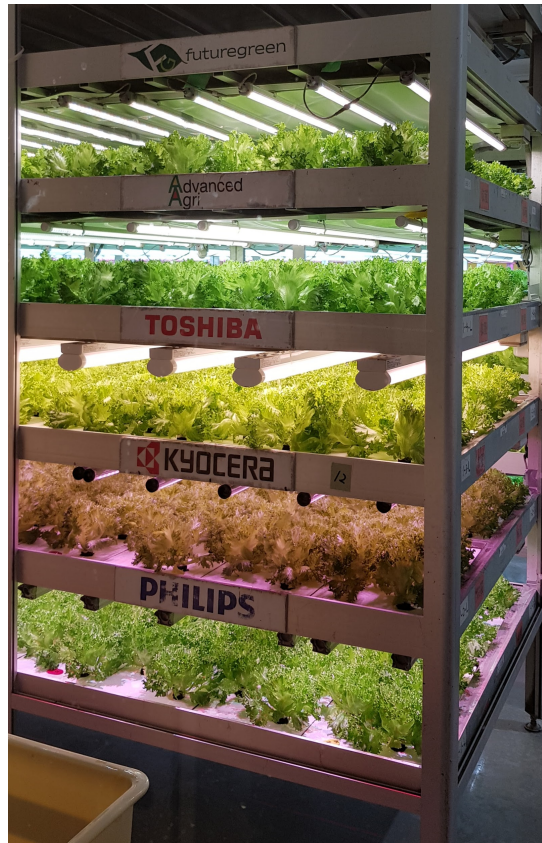
Figure 8. Testing rack of LED-technology from different suppliers (Source: Authors)
