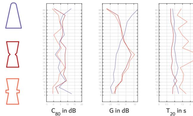
Moving the sound source. We expected that decreasing the length that the sound has to travel would improve the sound quality, but it also forces the sound to expand in a new direction. We choose to continue with hourglass (red) mainly due to loudness equality.
