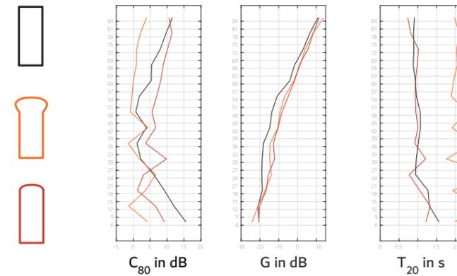
Evaluating the roof shapes effect on sound projection down through the room. The roundness of the roof must not be great enough to accumulate reverb (orange,  $T_{20}$ ), but project the sound early to help the clarity (red,  $C_{80}$ ).
