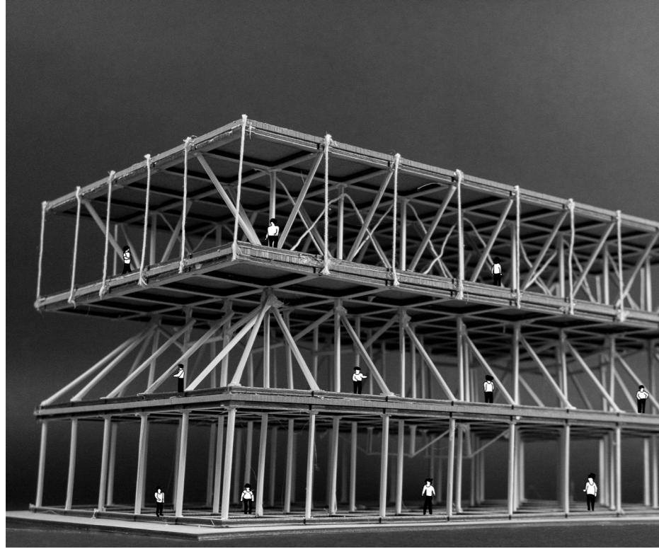
MODEL OF THE MAIN BUILDING'S STRUCTURAL SYSTEM WITH ANALYSIS MADE IN POINTSKETCH2D
