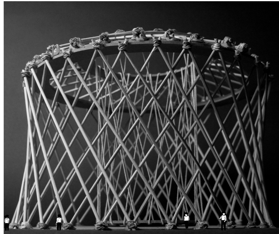
MODEL OF THE HELIX BUILDING'S STRUCTURAL SYSTEM WITH ANALYSIS MADE IN POINTSKETCH2D.
