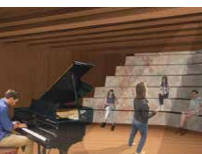
View 4: Interior view of the music recording studio showing the wood panels and non-parallel walls.
