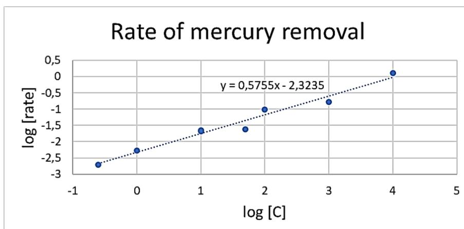
**Figure 4.4:** Calculated rate of mercury removal in the batch experiments versus the initial concentration.
