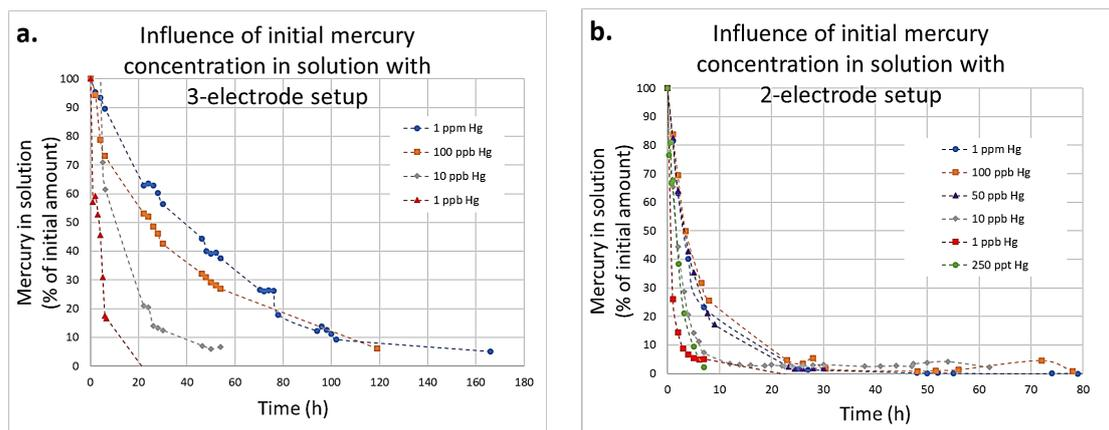
**Figure 4.2:** Graphs showing the decrease in mercury content in the electrolyte during batch experiments. All experiments with mercury dissolved in  $\text{HNO}_3$ . **a.** Experiments with three-electrode setup. Potential =  $-0.5$  V versus the reference electrode. **b.** Experiment with two-electrode setup. Potential =  $-1.81$  V versus the counter electrode.
