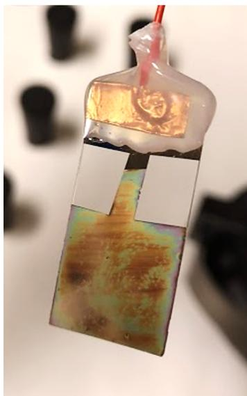
**Figure 4.6:** Working electrode that performed the 100 ppb Hg in tap water with a three-electrode setup. Potential = -0.91 V versus reference electrode.
