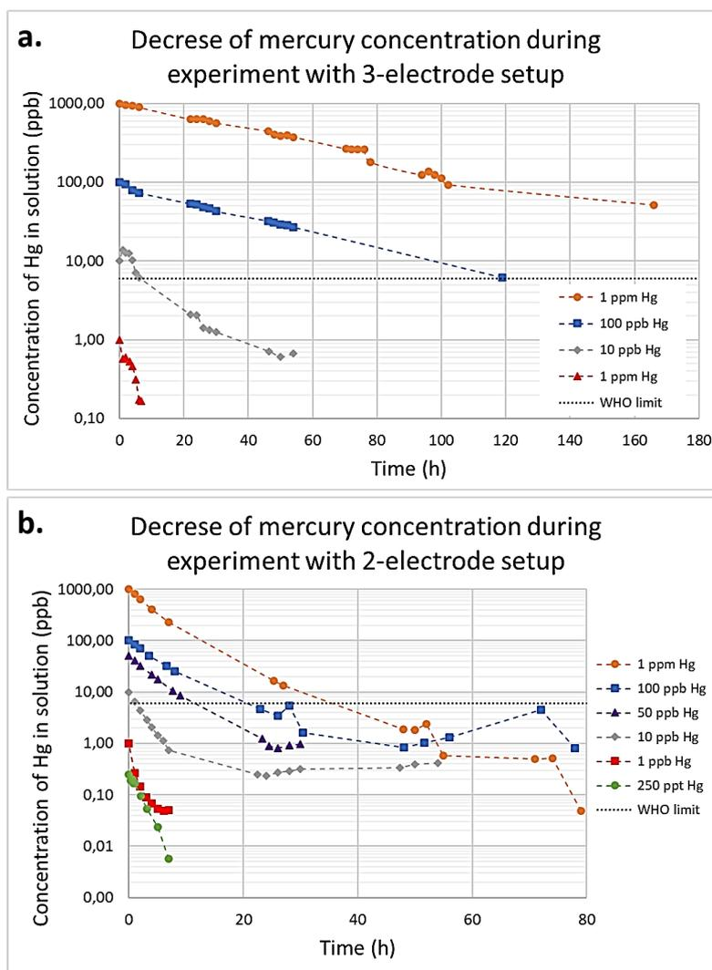
**Figure 4.3:** Graphs show the decrease in mercury concentration in the electrolyte during batch experiments. All experiments with mercury dissolved in  $\text{HNO}_3$ . **a.** Experiments with three-electrode setup. Potential =  $-0.5$  V versus reference electrode. **b.** Experiment with two-electrode setup. Potential =  $-1.81$  V versus counter electrode.
