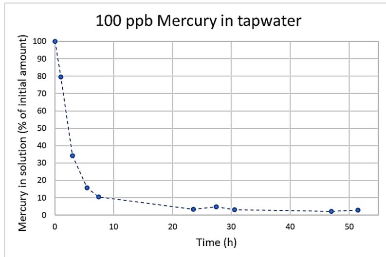
**Figure 4.7:** Graph showing the decrease in mercury content in the electrolyte during batch experiments. Electrolyte which consists of mercury dissolved in tap water. Potential =  $-0.91$  V vs. reference electrode.
