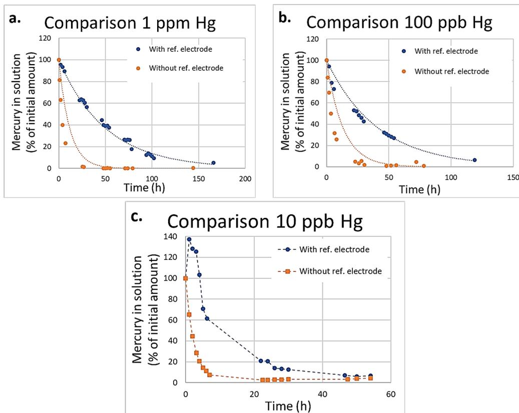
**Figure 4.1:** Graphs showing comparisons between using three-electrode and two-electrode setup. **a.** Comparison with initial electrolyte concentration of 1 ppm. **b.** Comparison with initial electrolyte concentration of 100 ppb. **c.** Comparison with initial electrolyte concentration of 10 ppb.
