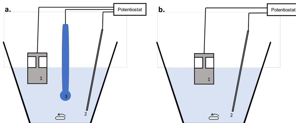
**Figure 2.1:** Sketch of the electrochemical cell set up. **a.** Three electrodes set up with a working electrode (1), a counter electrode (2) and a reference electrode (3). **b.** Two electrodes set up with a working electrode (1) and a counter electrode (2).
