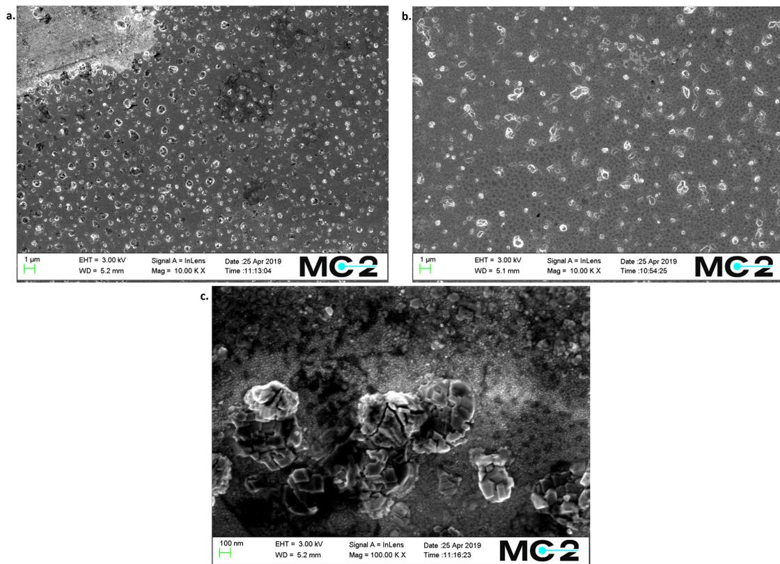
**Figure 4.5:** SEM pictures from the working electrode that preformed the 1 ppm Hg experiment with three-electrode setup. **a.** and **b.** are done with 3.0 kV and 10k magnification. **c.** are done with 3.0 kV and 100k magnification.
