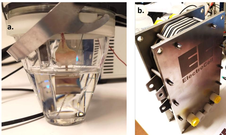
**Figure 3.2:** Experimental setups. **a.** Batch setup, 50 ml electrolyte, three-electrode configuration. **b.** The flow cell.
