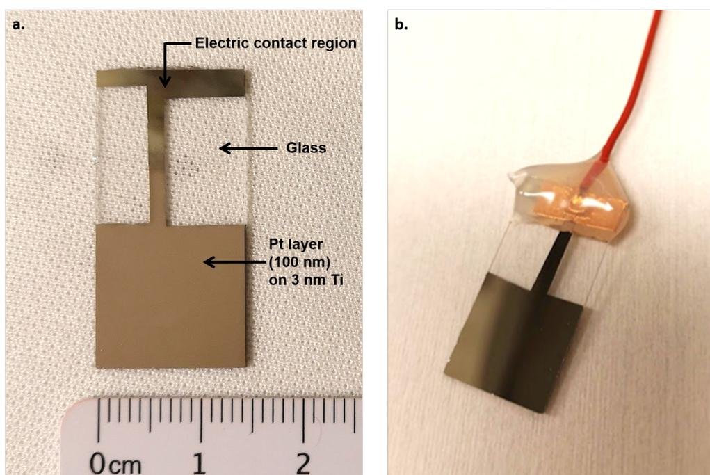
**Figure 3.1:** Working electrode. **a.** Design of the electrode, before the copper wire was attached. **b.** Completed electrode.
