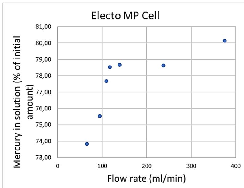
**Figure 4.8:** Amount of mercury still in solution after the experiment, versus the flow rate of the electrolyte.
