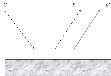
Figure 2.10: The variable G represent how well the material absorbs radiation from the surroundings. E represent how well the material emits thermal energy.
