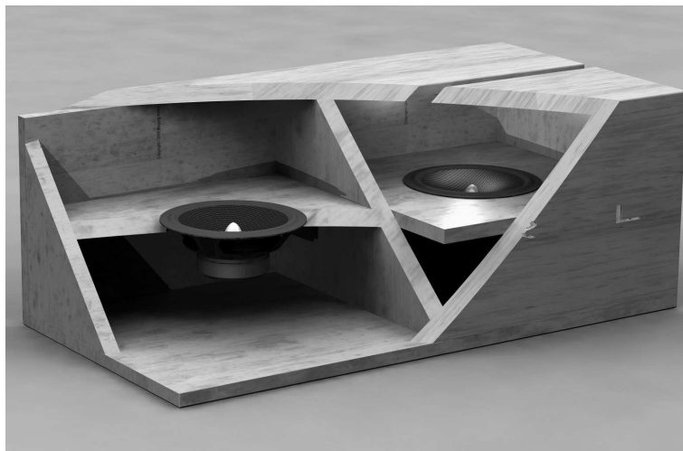
Figure 4.1. Illustration of the slit speaker.
