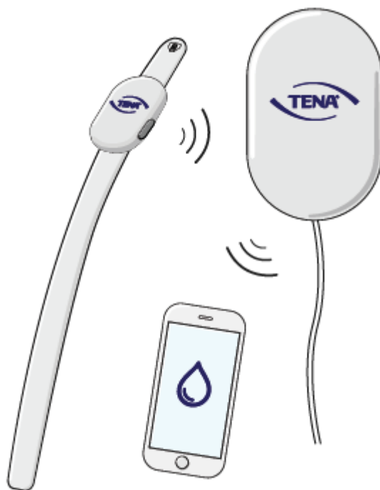
Figure 4: A graphical illustration of the physical TENA Change Indicator solution containing a strip with a logger which sends information to a gateway which presents the information on a smartphone.
