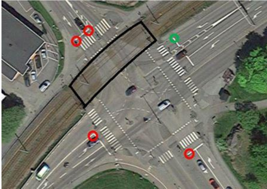
Figure 32 Improvement proposal for intersection 19. Black area represents the area of marking the tramway tracks with lines and different coating. Red circles are where warning signs for trams should be placed and green where the existing sign is located. Figure adjusted from Google maps (2019).
