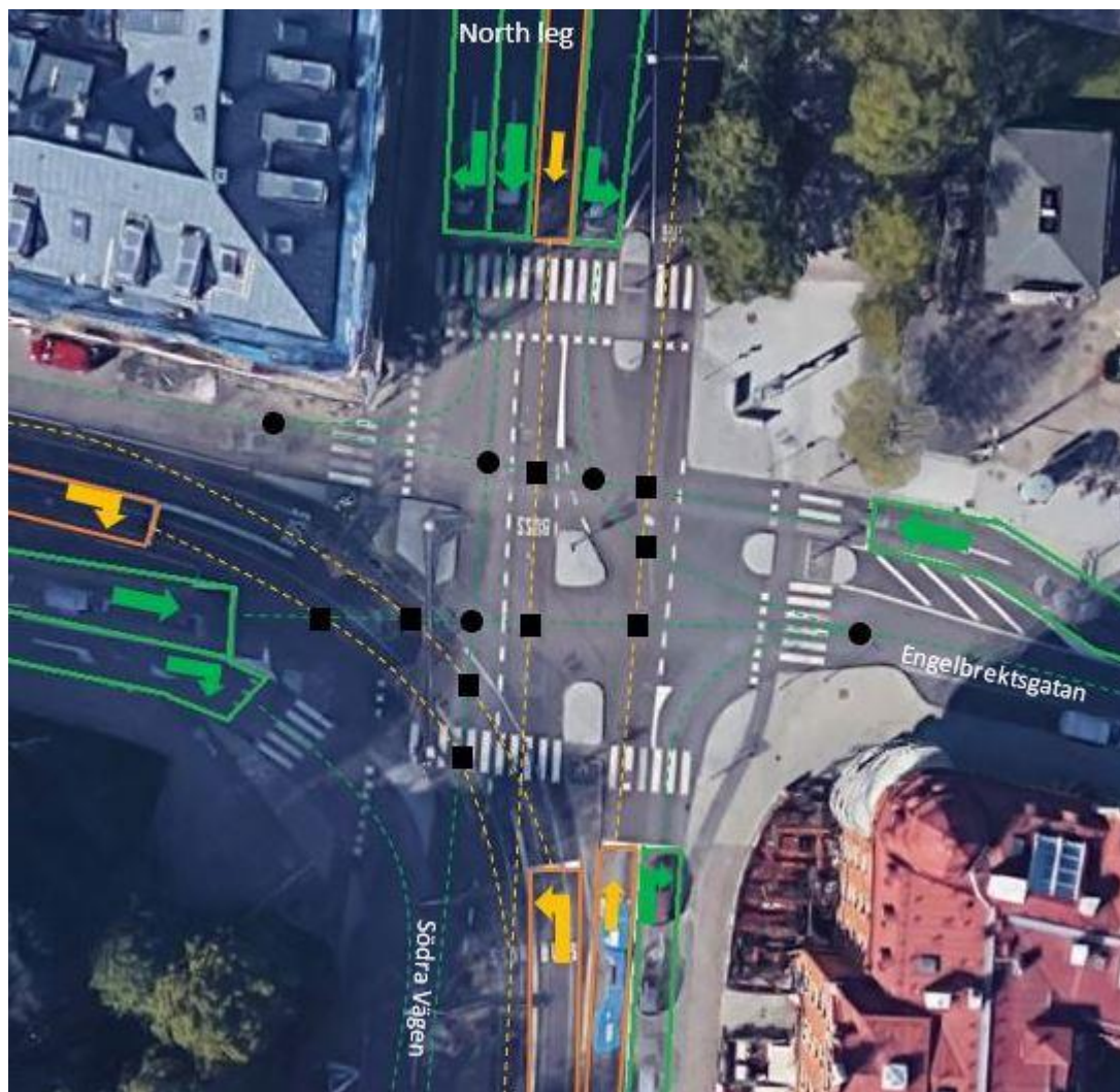
Figure 23 Map over intersection 7 marked with bus and tramway rail in orange and road in green. Theoretical conflict points marked by black circles for private vehicle-private vehicle conflict and black squares for private vehicle-public transport conflicts. Figure adjusted from Google maps (2019).
