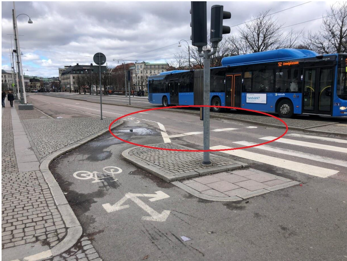
Figure 27 North leg of intersection Nya Allén/Kungsporsavenyen. The red marking represents the area where the bike box should be placed, by withdrawing the stop line for vehicles and making the cyclists stop in front of the vehicles. Author's own copyright.
