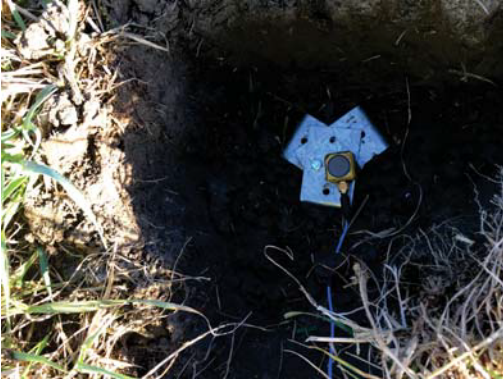
Figure 5.4.: Mounting of accelerometer
