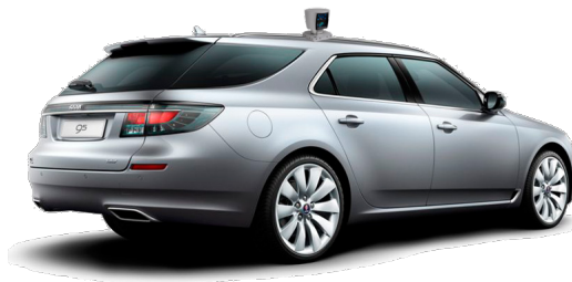
Figure 1.1: Car with a LIDAR mounted on its roof
