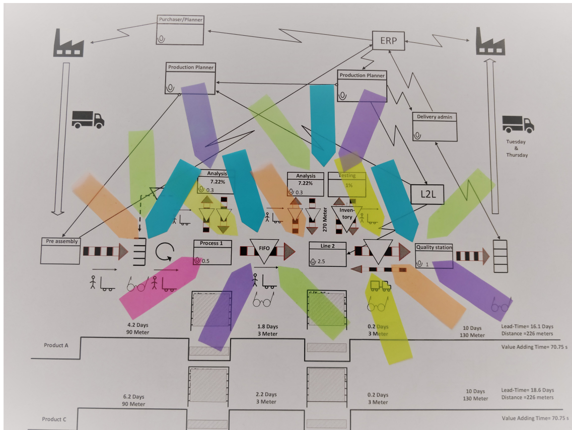
Figure A.2: Identified problems of sensor flow in Assembly 1
