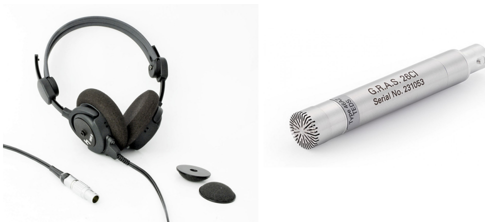
Figure 3.2: BHS II - binaural headphone (HEAD acoustics GmbH, 2018b) & GRAS microphone (GRAS Sound & Vibration A/S, 2018)
