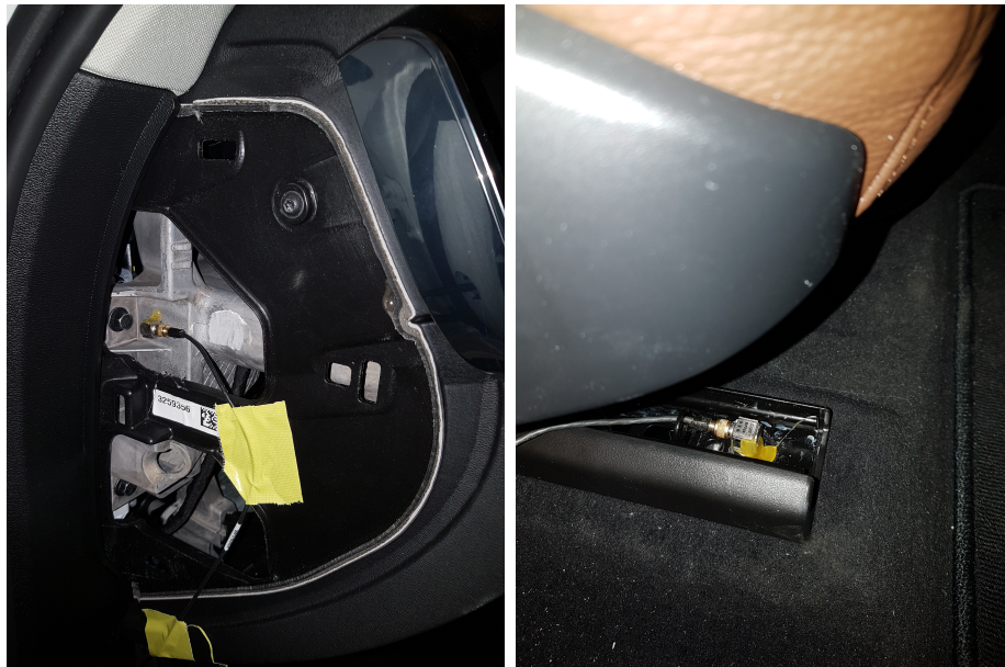
Figure 3.13: Accelerometer on the instrument panel and seat rail
