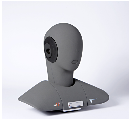
Figure 3.4: HEAD Measurement System - HMS IV - Acoustic Head (HEAD acoustics GmbH, 2018a)
