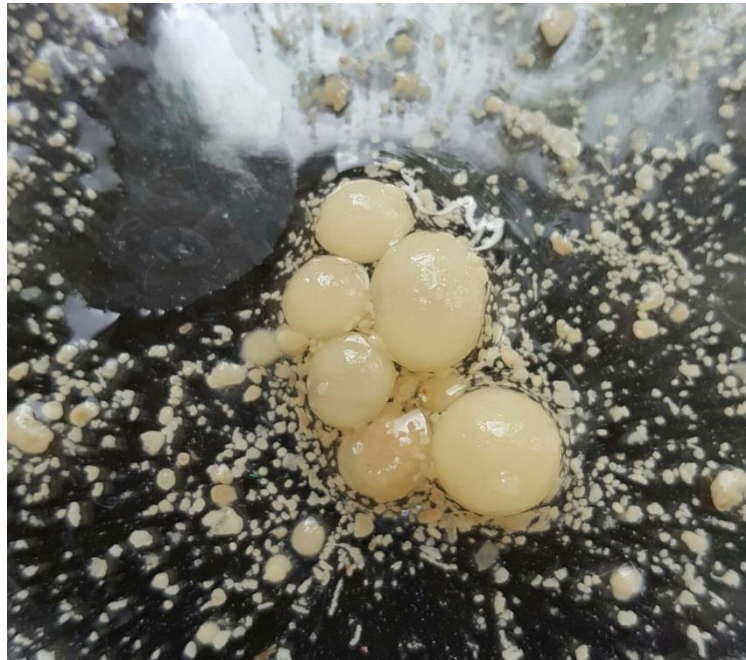
Figure 0-3. Aerobic granular sludge
