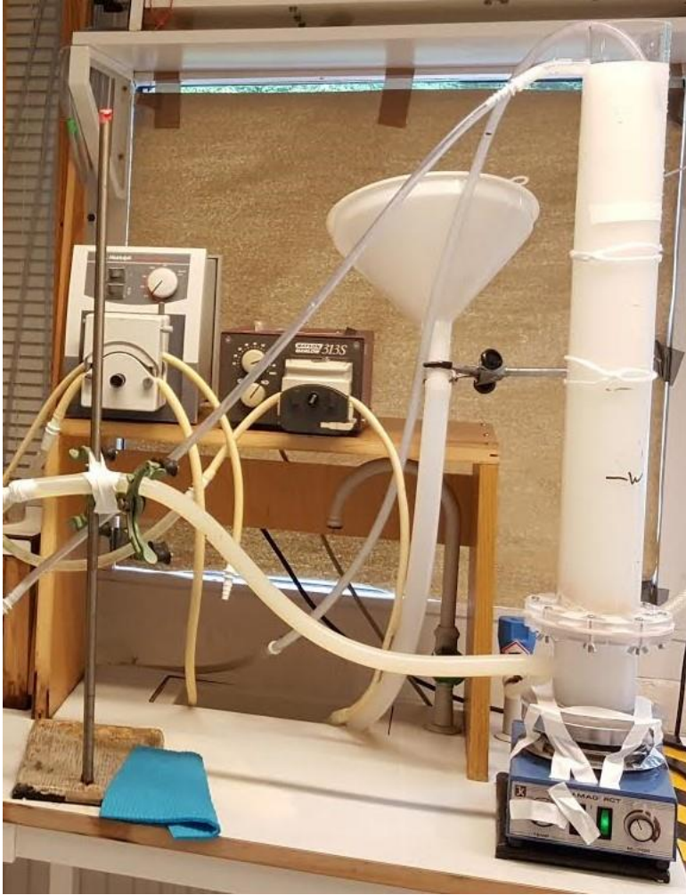
Figure 0-12. Kaolin suspension (in the filter column) and the installations
