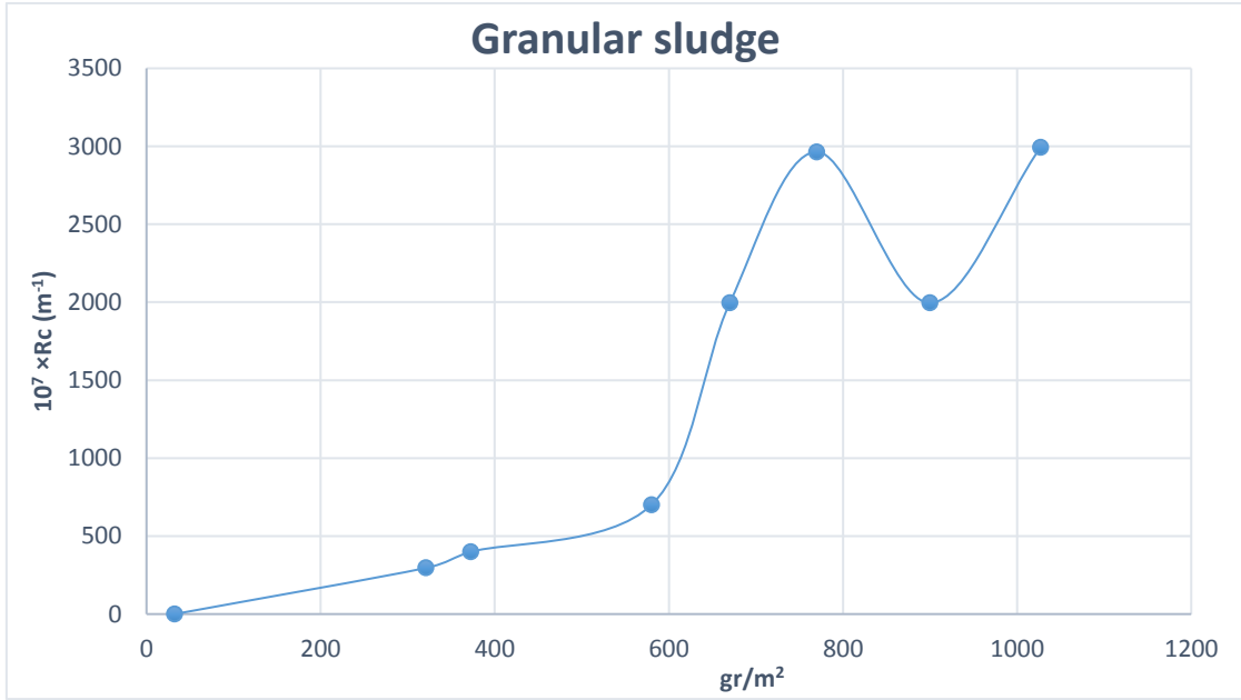
Figure 0-61. Cake layer resistance for sludge from R3 per square meter of the membrane (first trial)
