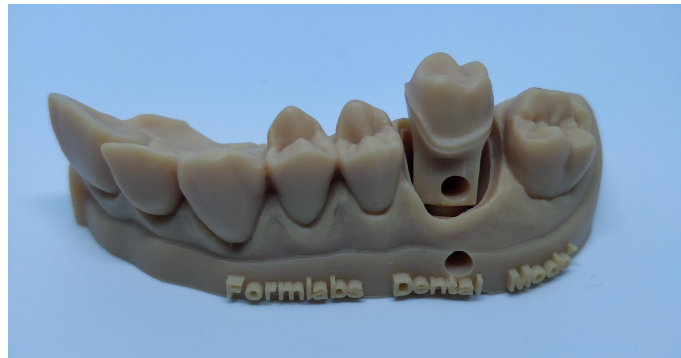
Figure 3.3: Picture of a 3D-printed study model, printed from a Formlabs file (photo taken by authors)
