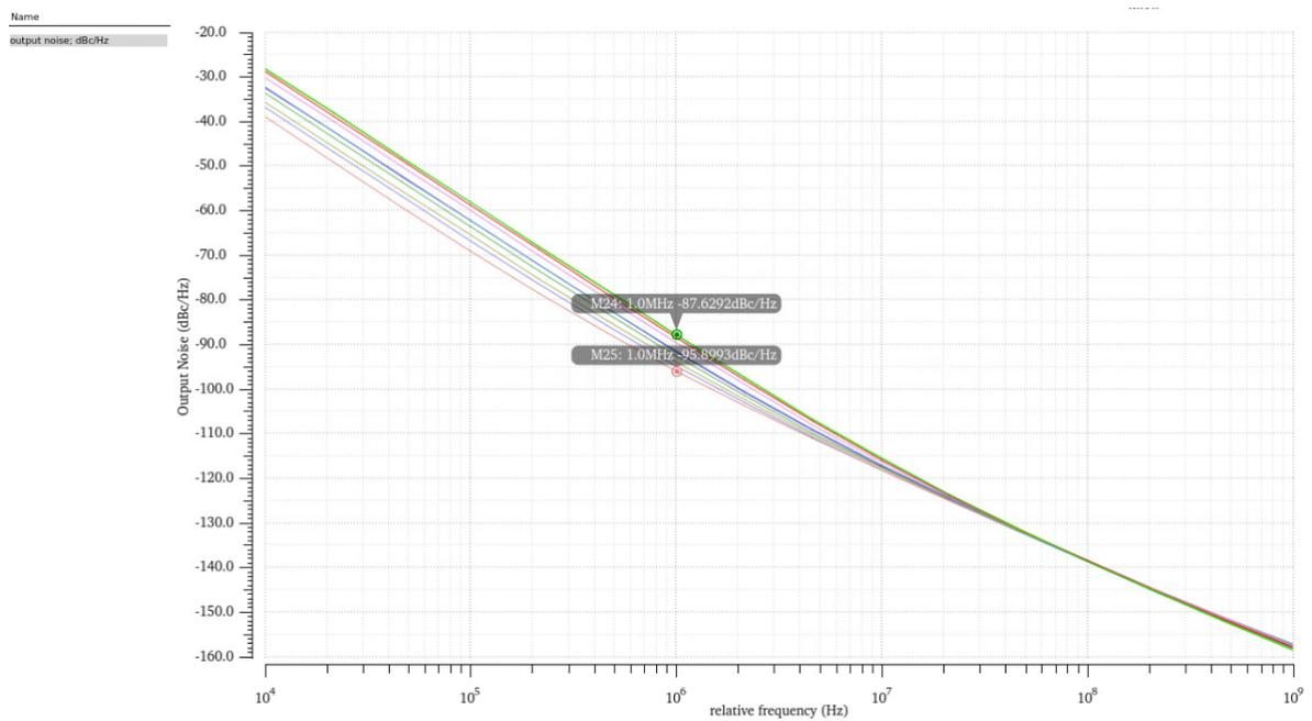
Figure 4.6: Phase noise in ILFD output
