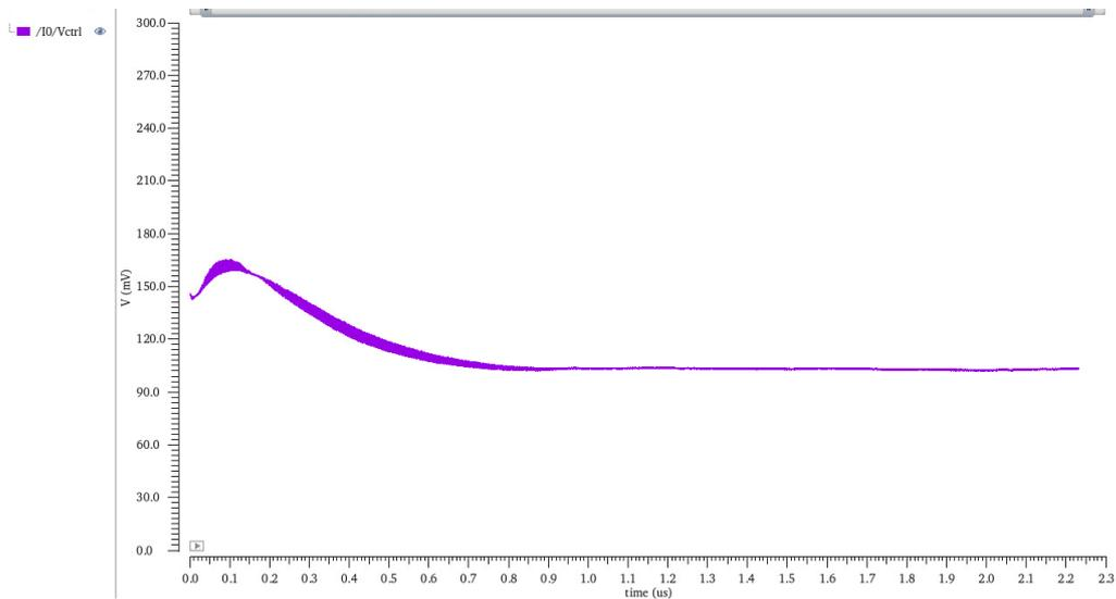
**Figure 4.11:** PLL control voltage at the input of VCO
