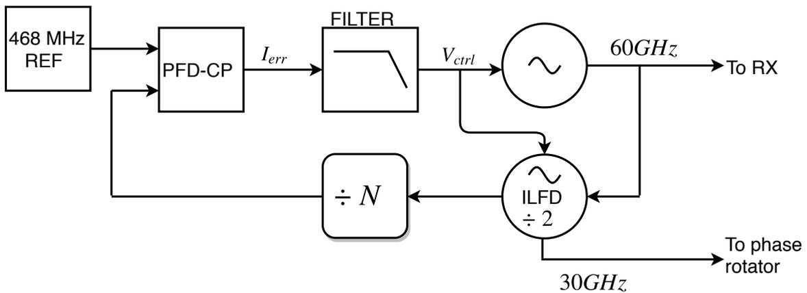
**Figure 1.4:** Basic PLL block diagram
