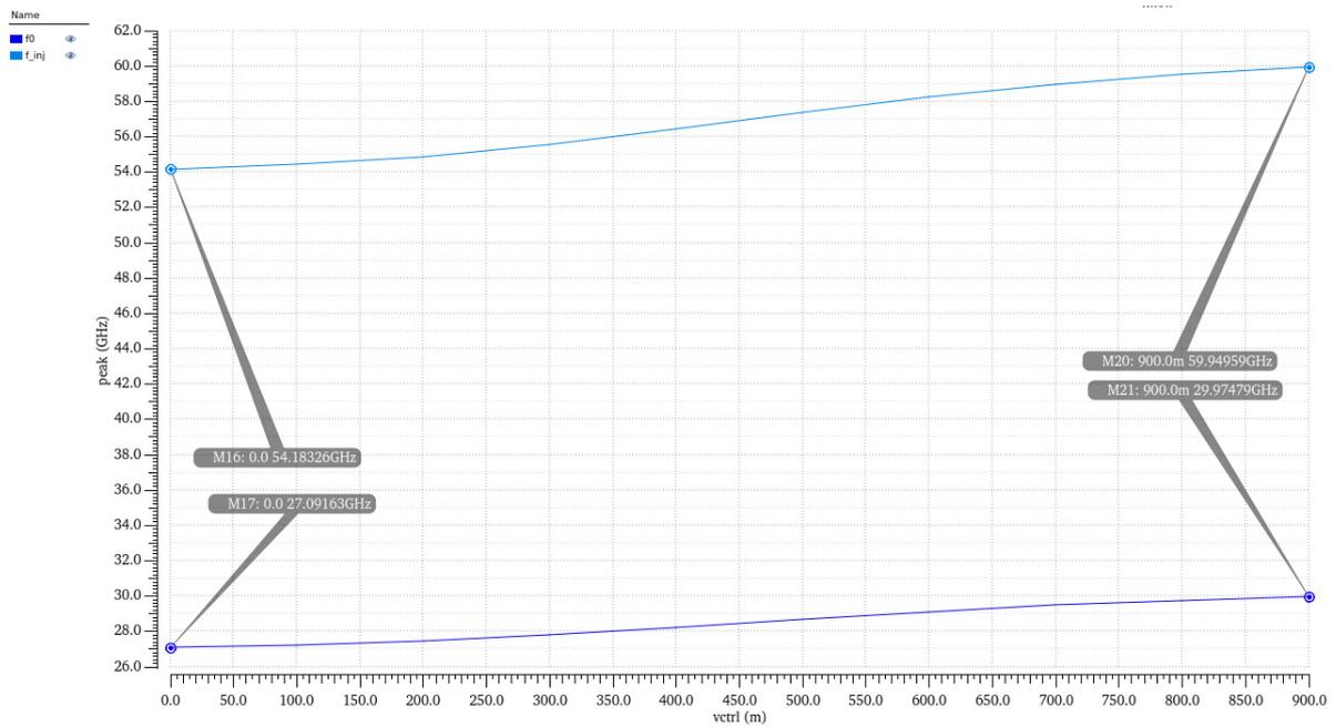
Figure 4.5: Tuning of ILFD and VCO frequency by control voltage variation
