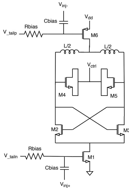
**Figure 2.5:** Injection Locked Frequency Divider
