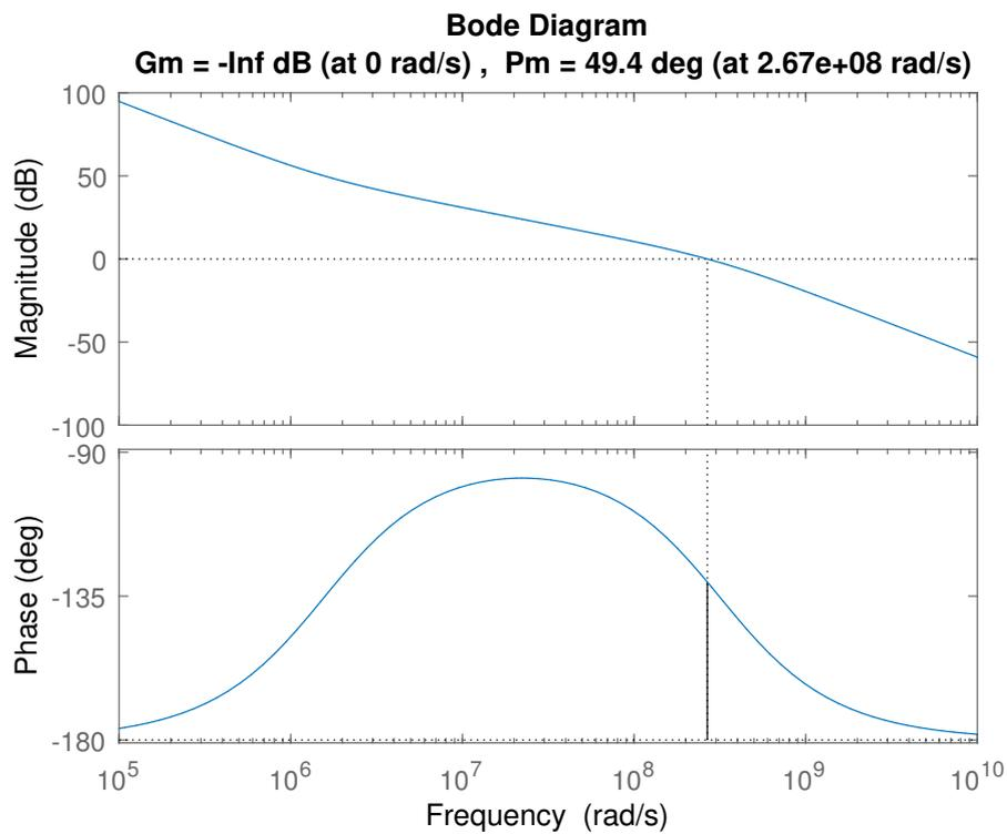
Figure 4.2: PLL open loop response
