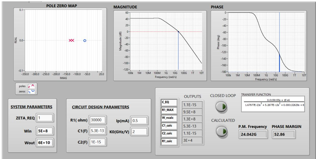
Figure 3.1: PLL system design GUI in LabVIEW
