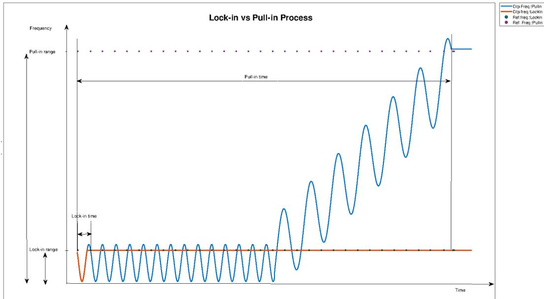
Figure 2.1: Lock-in and Pull-in process
