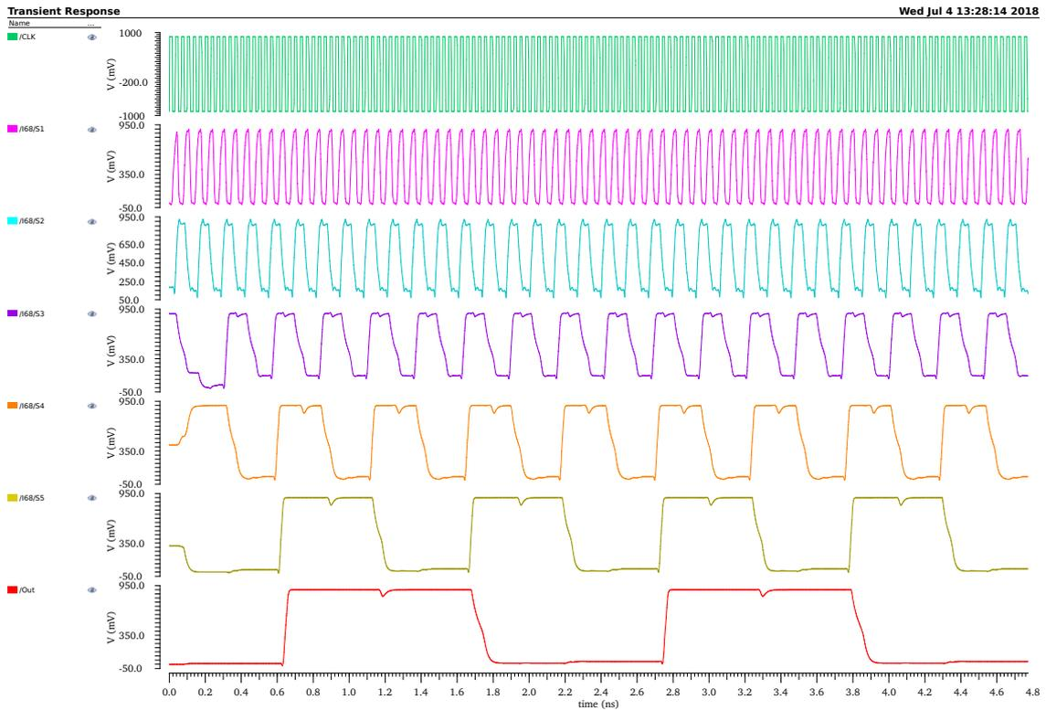
**Figure 4.8:** Divider chain waveforms (With keeper): Input clock and stages 1 to 6 output waveforms
