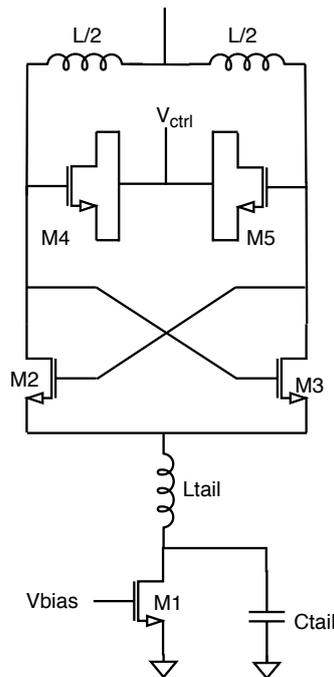
**Figure 2.3:** Voltage Controlled Oscillator
