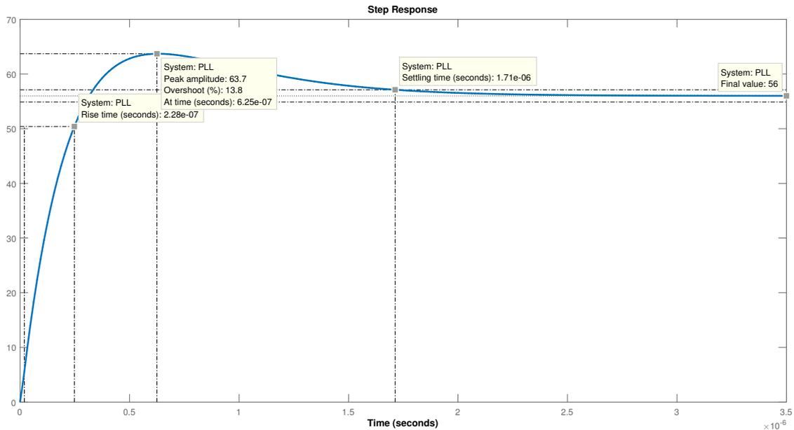
**Figure 4.3:** PLL system step response
