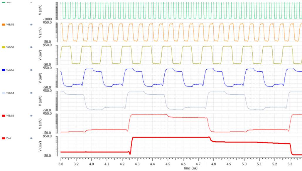
**Figure 4.7:** Divider chain waveforms (Without keeper): Input clock, stages 1 to 6 output waveforms
