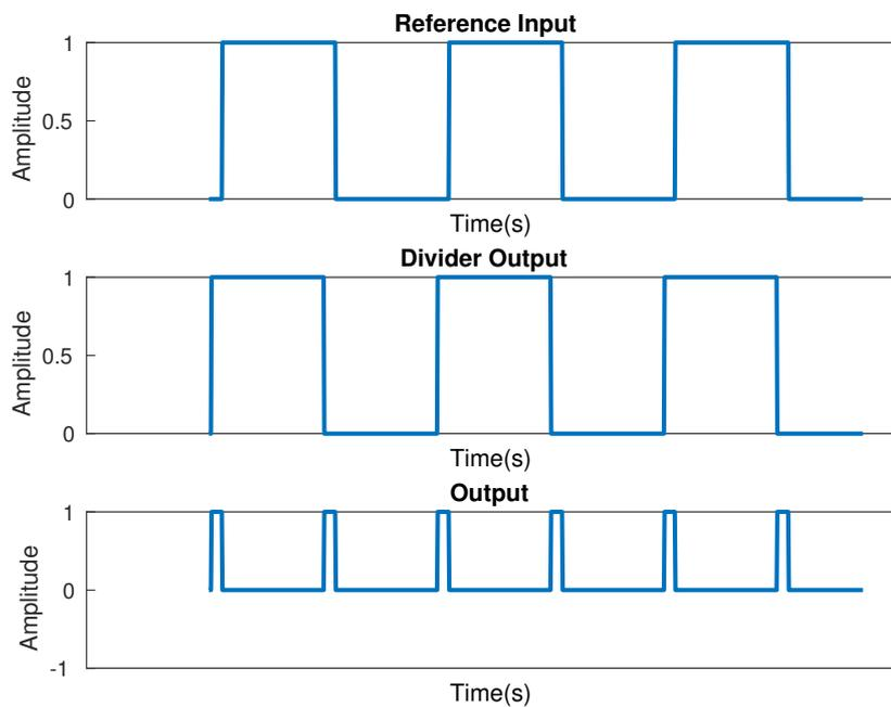
**Figure 2.10:** PFD output and input waveforms:  $freq_1 = freq_2$ ,  $\phi_1 > \phi_2$
