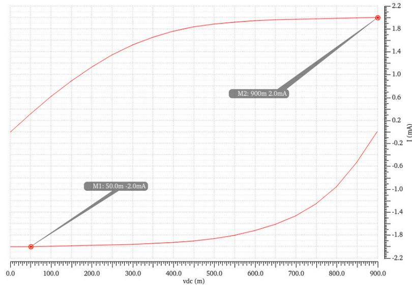
**Figure 4.9:** Charge pump current for Up (top) and Down (bottom) signals activated
