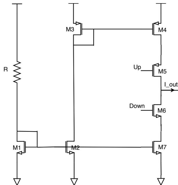
Figure 2.14: Charge Pump Circuit
