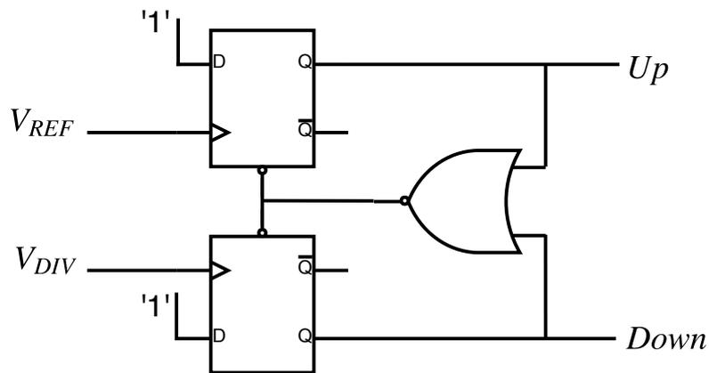
**Figure 2.9:** Phase Frequency Detector block diagram
