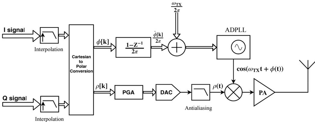
**Figure 1.2:** An example polar transmitter architecture[3] utilizing digital PLL
