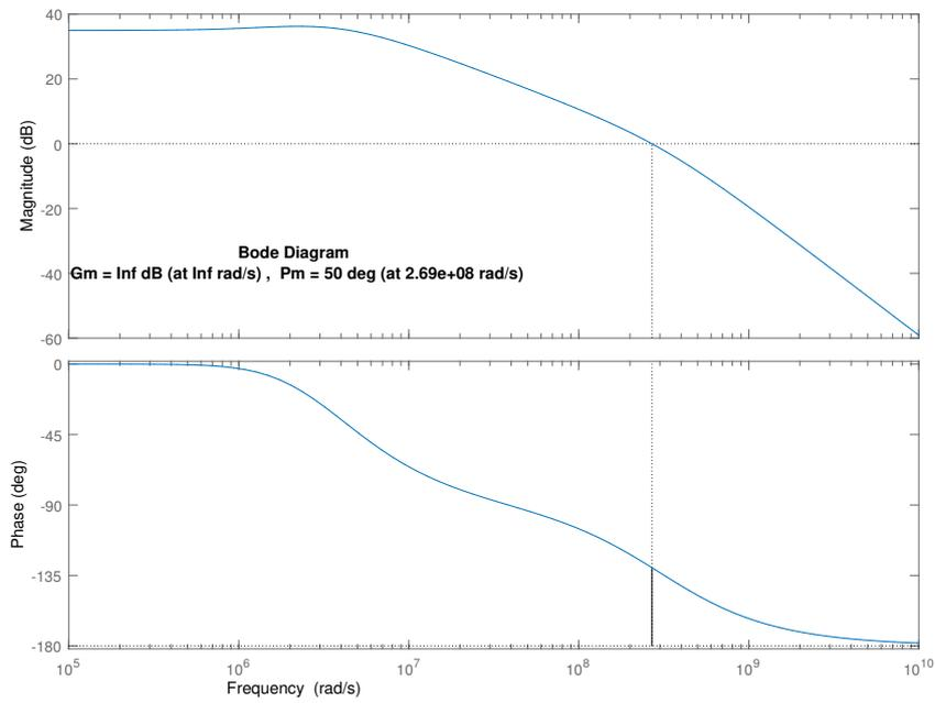
Figure 4.1: PLL closed loop response
