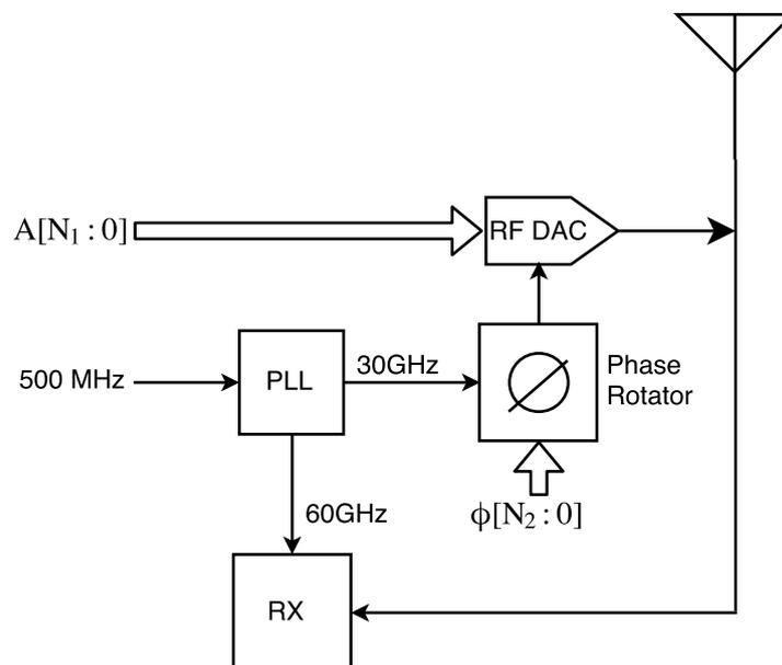
**Figure 1.3:** Polar Transceiver architecture with baseband direct conversion
