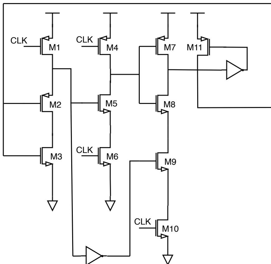
**Figure 2.8:** Keeper circuit added to TSPC based divider[21]
