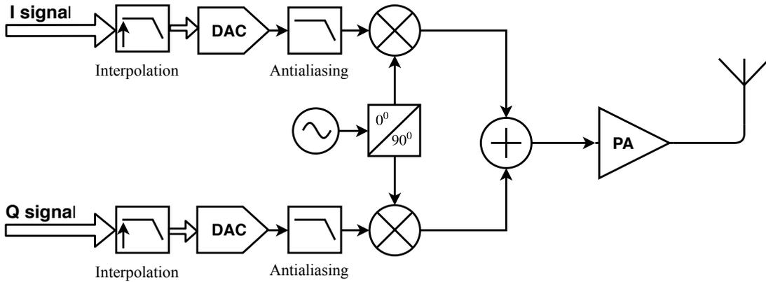
**Figure 1.1:** An example IQ transmitter architecture with baseband direct conversion[3]
