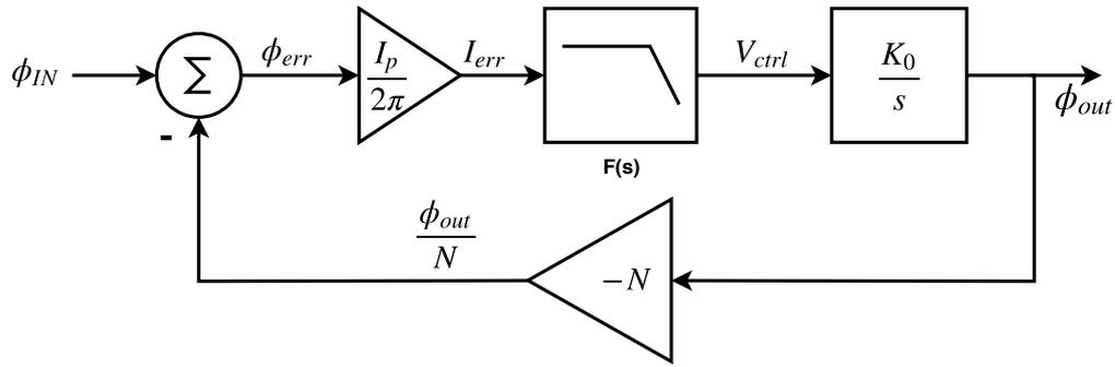
**Figure 2.2:** Linear Phase Model of PLL
