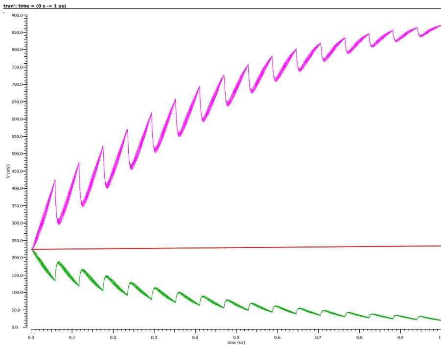
**Figure 4.10:** Control Voltage for  $f_{div} < f_{ref}$  (Pink) b.  $f_{div} = f_{ref}$  (Red) c.  $f_{div} > f_{ref}$  (Green)
