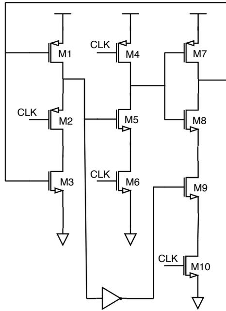
**Figure 2.6:** TSPC schematic 1
