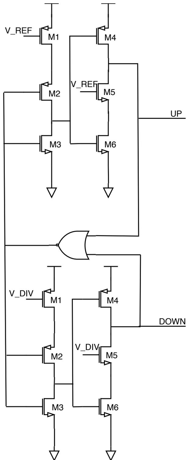
**Figure 2.13:** Phase Frequency Detector circuit
