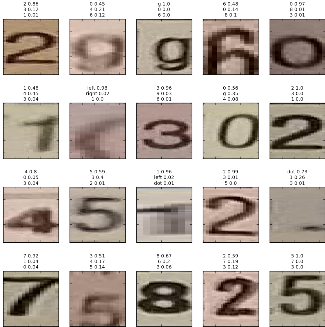
Figure 4.5: 20 samples of the classification of the images in the validation set. Top three classifications and the corresponding probabilities are listed. The algorithm classifies most characters correctly.
