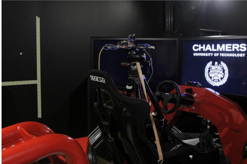
Figure 4.11: The test rig placed on a  $6DOF$  platform for testing
