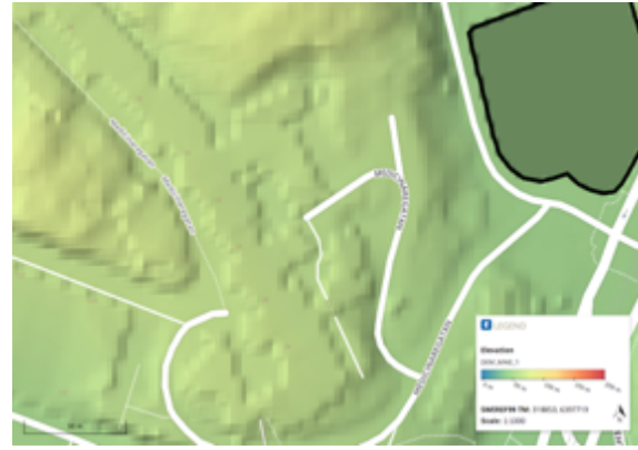
Figure 4-33: DEM model in SCALGO with 4x4 m raster of MIKE ZERO for area around Sahlgrenska University Hospital (created by author)
