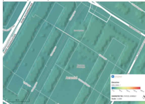
Figure 4-35: DEM model in SCALGO with 4x4 m raster of MIKE ZERO for Annedal area (created by author)
