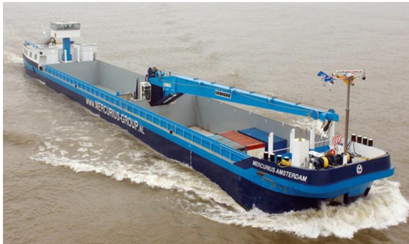
Picture 5, Sample IWW vessel with crane suitable for container operation in all ports in the Lake.
