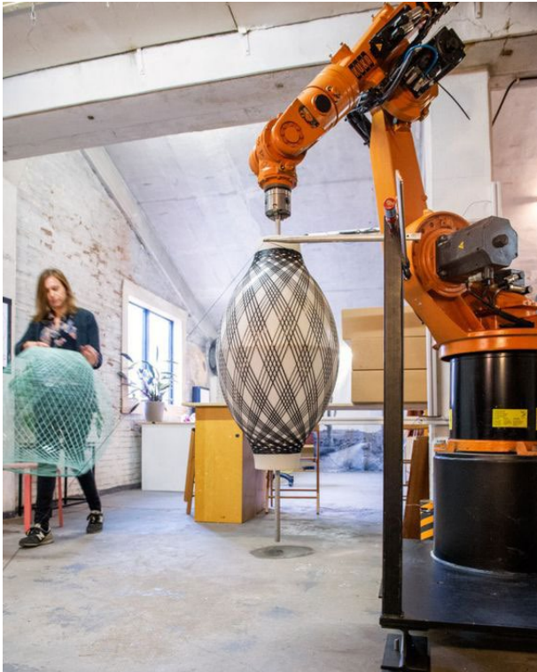
Figure-16. A Lamp Made with the Help of a Robot (Laupman & Musial, 2015). Reprinted with permission.
