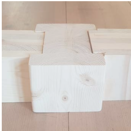
This was an early idea for the wall construction, made out of CLT. In the final version the CLT was replaced by Iso-timber.
