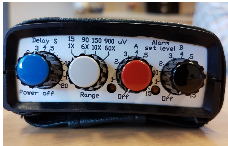
Figure 2.7: An EMG amplifier unit using at SÄS. Gains can be adjusted by the white knob and threshold level can be selected by the red and black knob for channel A and channel B respectively. The blue knob is used for adjusting the delay in a unit of second(s).
