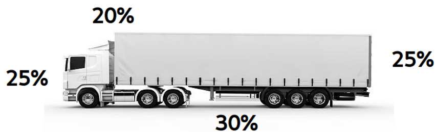
Figure 2.3: Distribution of aerodynamic drag for a heavy vehicle tractor-trailer truck.
