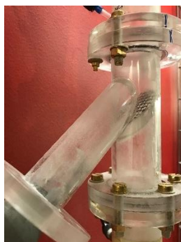
Figure 4.5. Extension arm after the cyclone with a net that collect the particles
