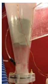
Figure 4.11. Slugging phenomenon in the cyclone
