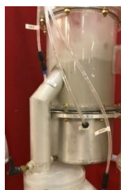
Figure 4.12. Bed material accumulated in the arm between the fuel reactor ant the post-seal
