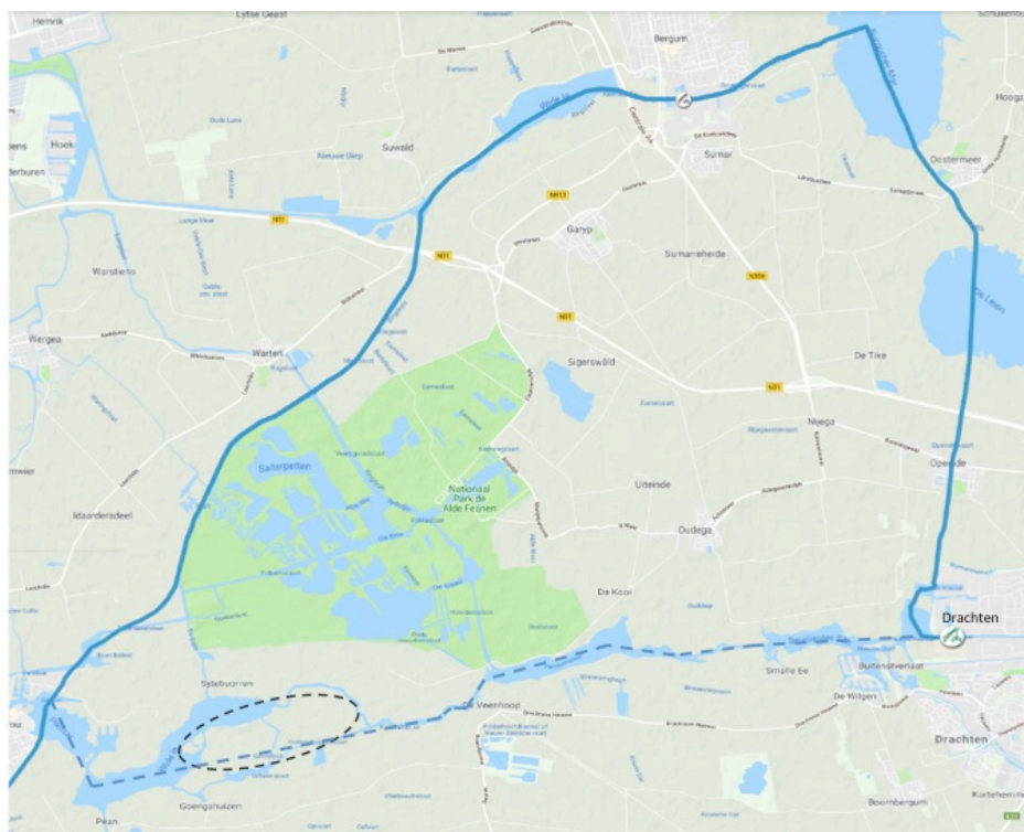
Figure 7. Waterways in Drachten. The solid line represents the current waterway, whereas the dashed line is where the new class V waterway would be. The circled area is the wetland that would be integrated in the waterway (Blue Road Map, 2018, edited by authors).
