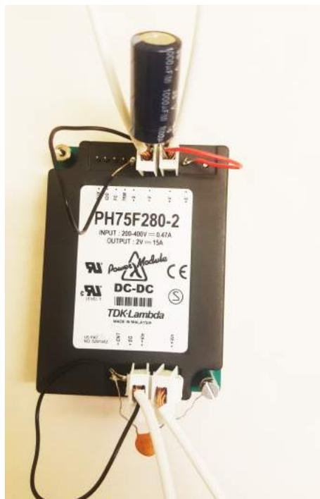
Figure 5.14: DC-DC converter.
