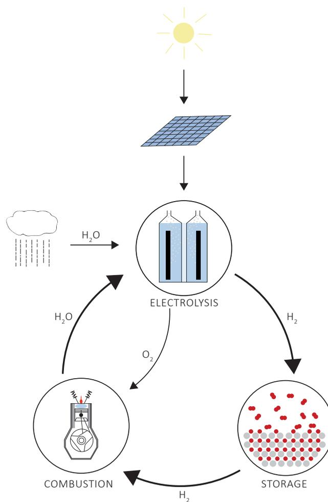
**Figure 3.1:** The hydrogen cycle: water is split into hydrogen gas which is stored and then used.
