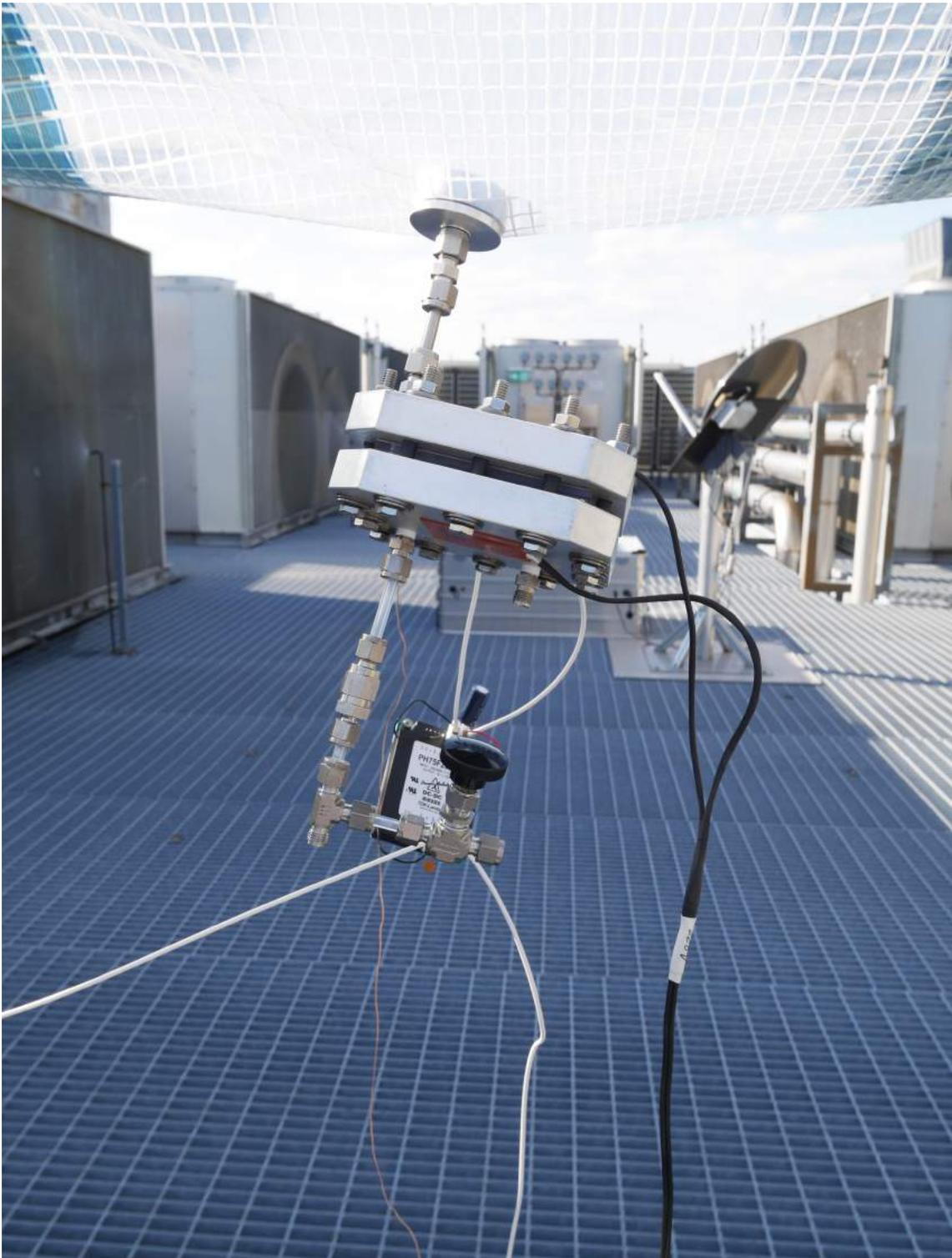
**Figure 5.20:** Electrolyzer connected to the solar roof.
