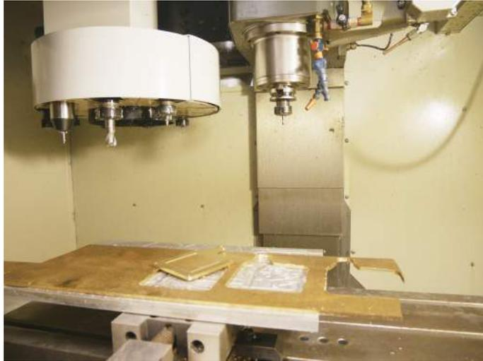
**Figure 5.9:** CNC-milling of flow field plates.
