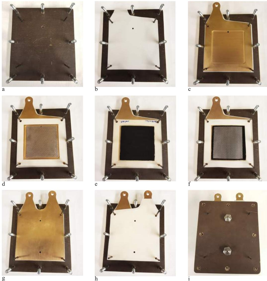
**Figure 5.13:** Assembling the electrolyzer step by step.
