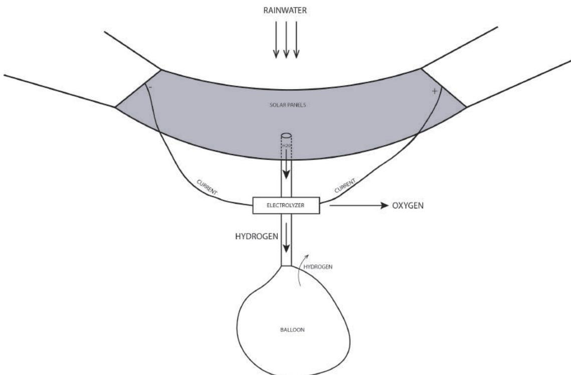
**Figure 5.15:** Sketch of prototype.
