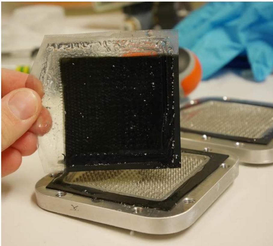
**Figure 5.6:** MEA after running electrolysis, electrolyzer 1.
