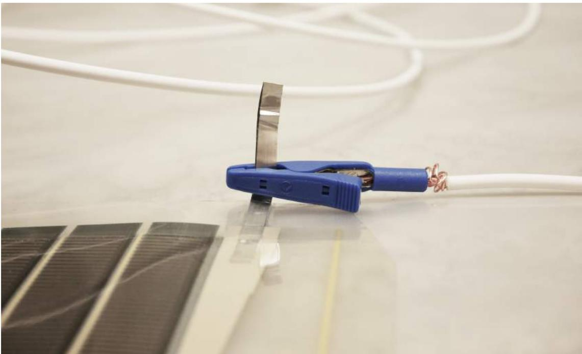
**Figure 5.17:** Connection between solar panel and cable.
