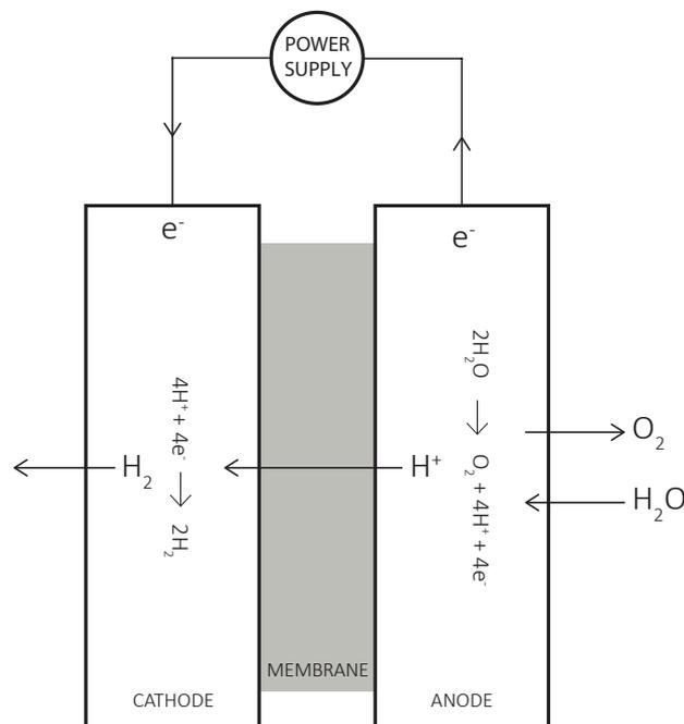
**Figure 3.2:** PEM electrolysis.
