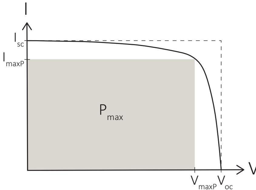
**Figure 5.2:** Maximum current and voltage.
