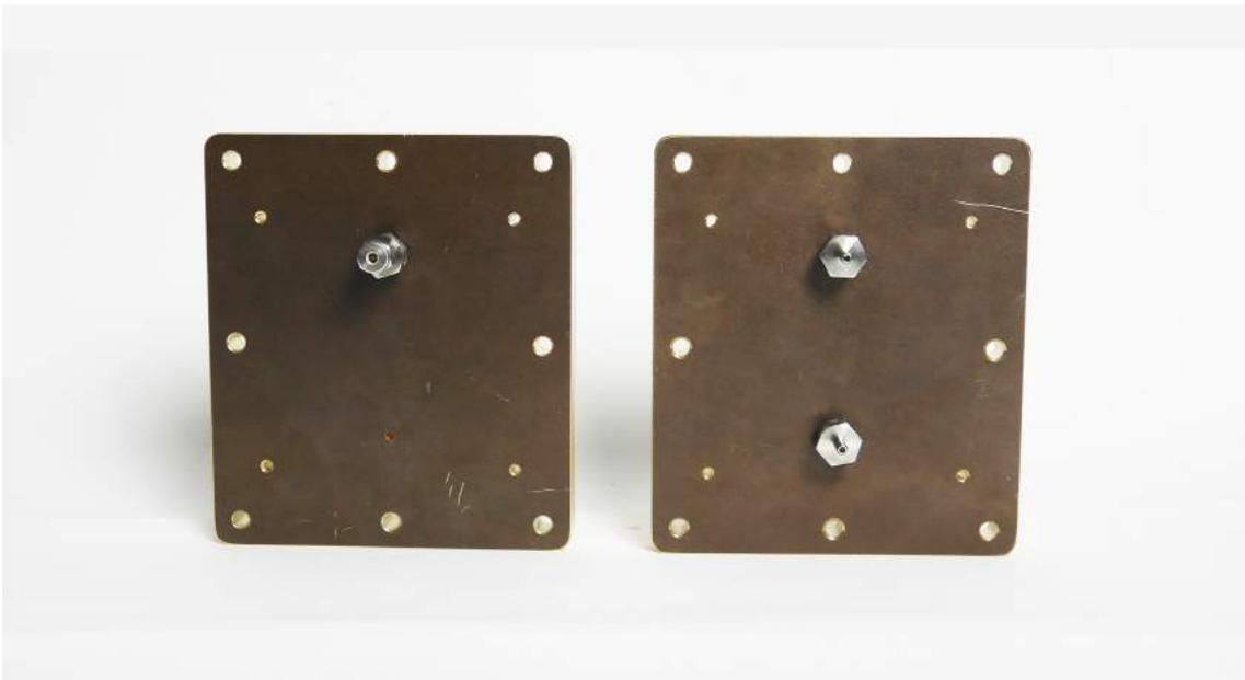
**Figure 5.7:** End plates with connections for water, oxygen and hydrogen gas.
