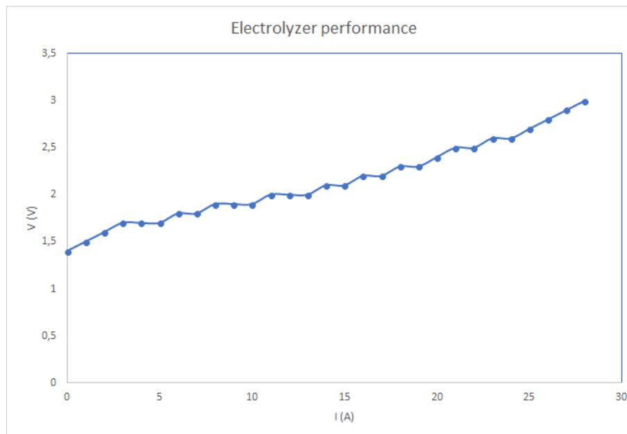
**Figure 6.1:** Voltage as a function of current.
