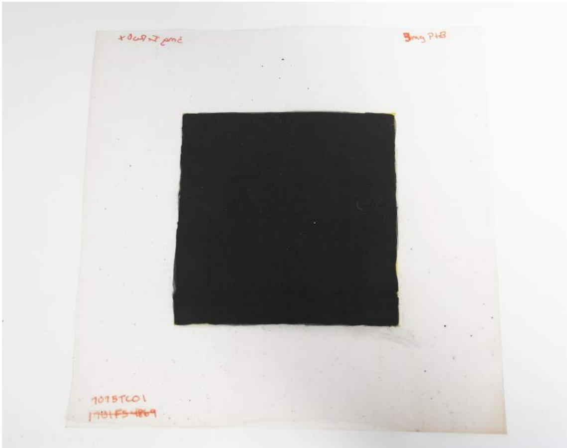
**Figure 5.12:** Electrolyzer MEA, electrolyzer 2.
