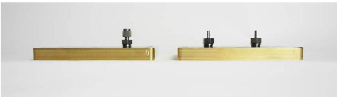
**Figure 5.8:** End plates electrolyzer 2.
