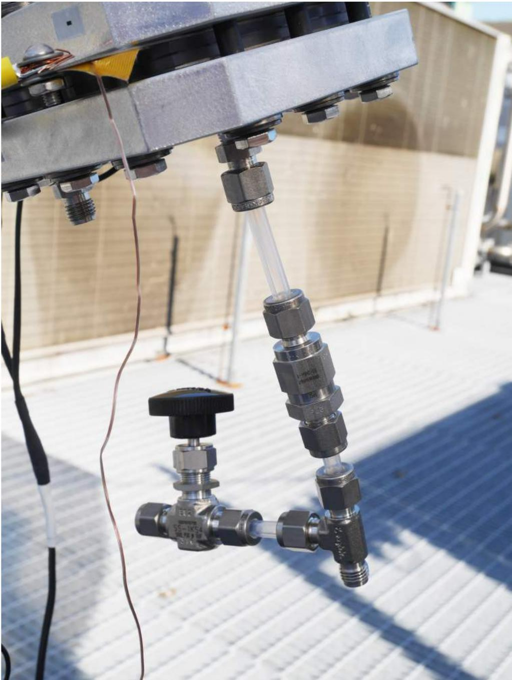
**Figure 5.21:** Tap for hydrogen to exit the weather balloon.
