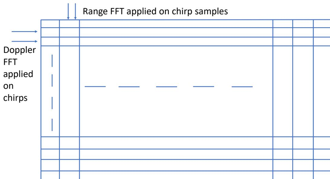
**Figure 2.5:** Structure of the digitized signal and how two dimensional FFT performs. Range FFT held on column wise for the chirp samples and Doppler FFT held row-wise for the reflected chirps.
