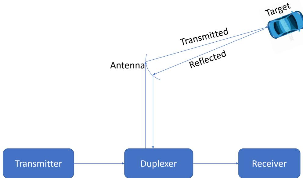
**Figure 2.1:** General simplified block diagram of radar systems.
