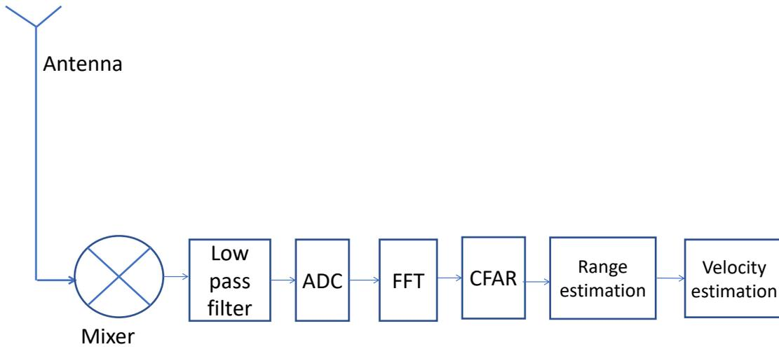
**Figure 2.3:** General receiver block diagram for FMCW radars.
