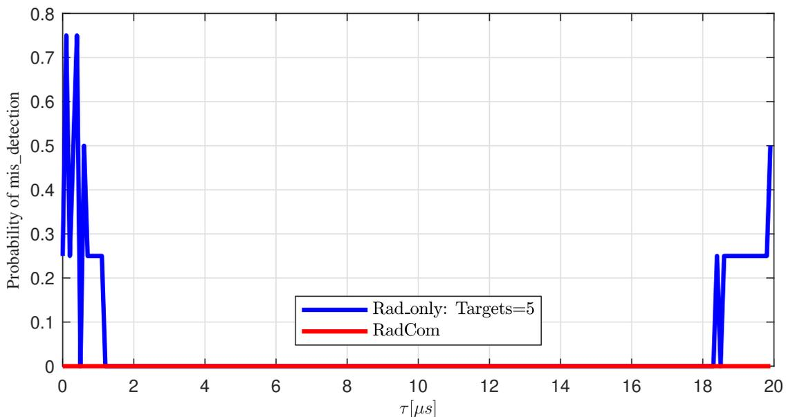
**Figure 5.1:** Probability mis-detection of target with and without RadCom systems. The simulation contains four other interfering targets besides the ego target and the threshold value is  $10dB$ .
