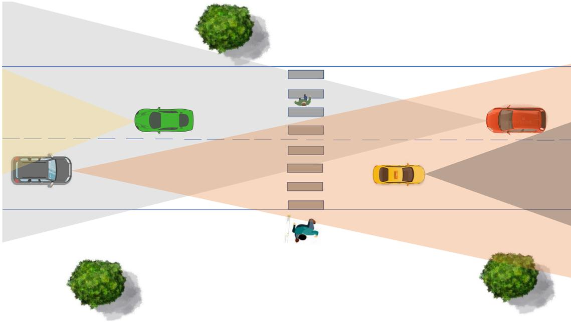
**Figure 1.1:** Mutual interference of signals from four cars with front side radars and including pedestrian line for passengers.
