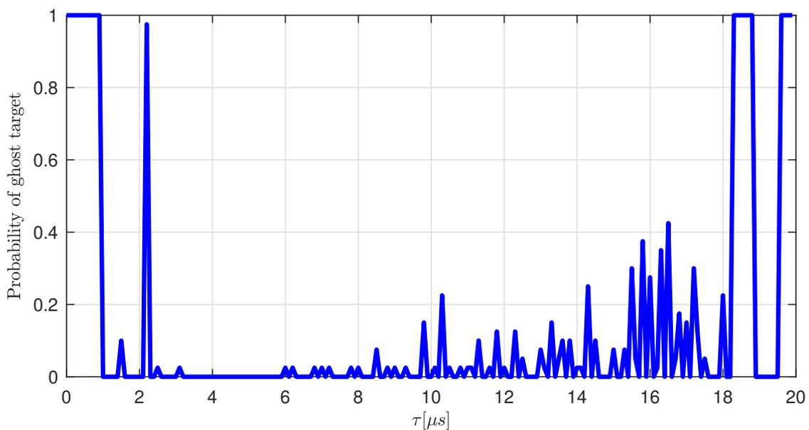
**Figure 5.4:** Probability of ghost target detection using radar only systems. The simulation contains four other interfering targets besides the ego target and the threshold value is  $7dB$ .
