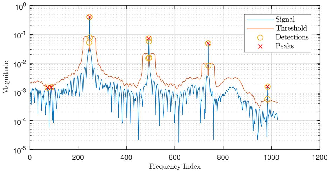
**Figure 5.6:** Target detection from output of the FFT signal using the implemented CFAR and the threshold value is  $7dB$ . We have more four interfering targets beside the ego vehicle.
