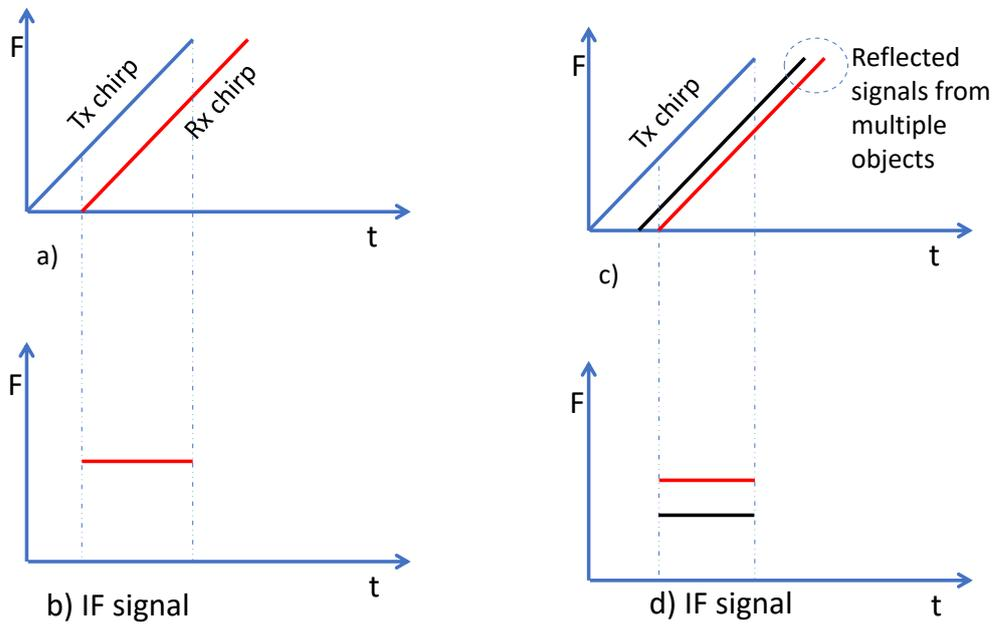
**Figure 2.7:** IF signal and IF frequency spectrum of received signal in dB from one and two reflections.
