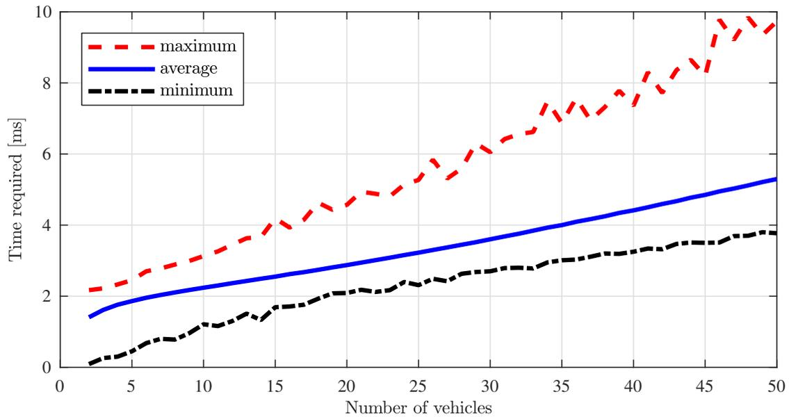
**Figure 5.9:** The required time for resolving the communication contention among the vehicles in RadCom using  $B_c = 40$  MHz, P-persistent CSMA without back off.
