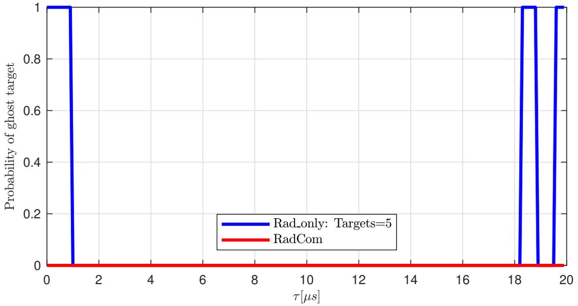
**Figure 5.2:** Probability of ghost target detection with and without RadCom systems. The simulation contains four other interfering targets besides the ego target and the threshold value is  $10dB$ .
