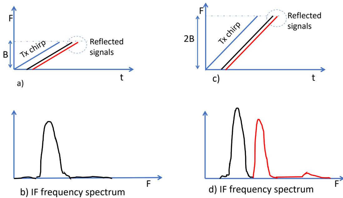
**Figure 2.10:** Importance of bandwidth in determining range resolution.
