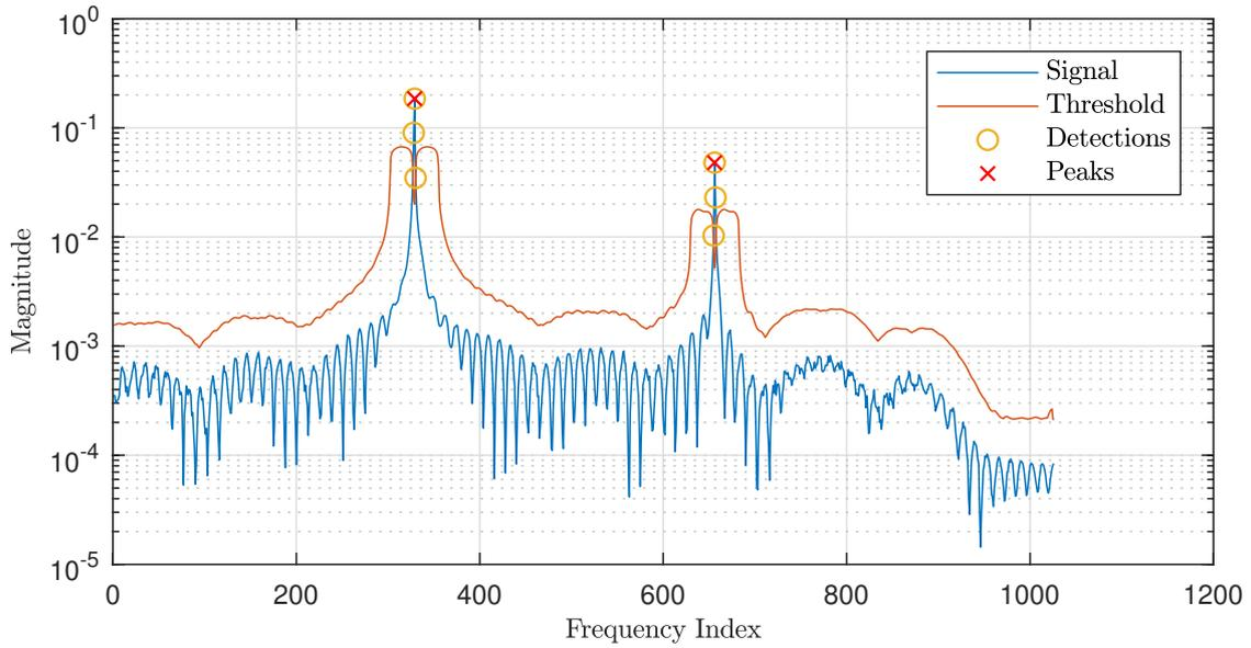
**Figure 2.6:** CFAR detection using 10dB threshold on out of the range FFT. We have two targets at 50m and 100m from the FMCW radar.
