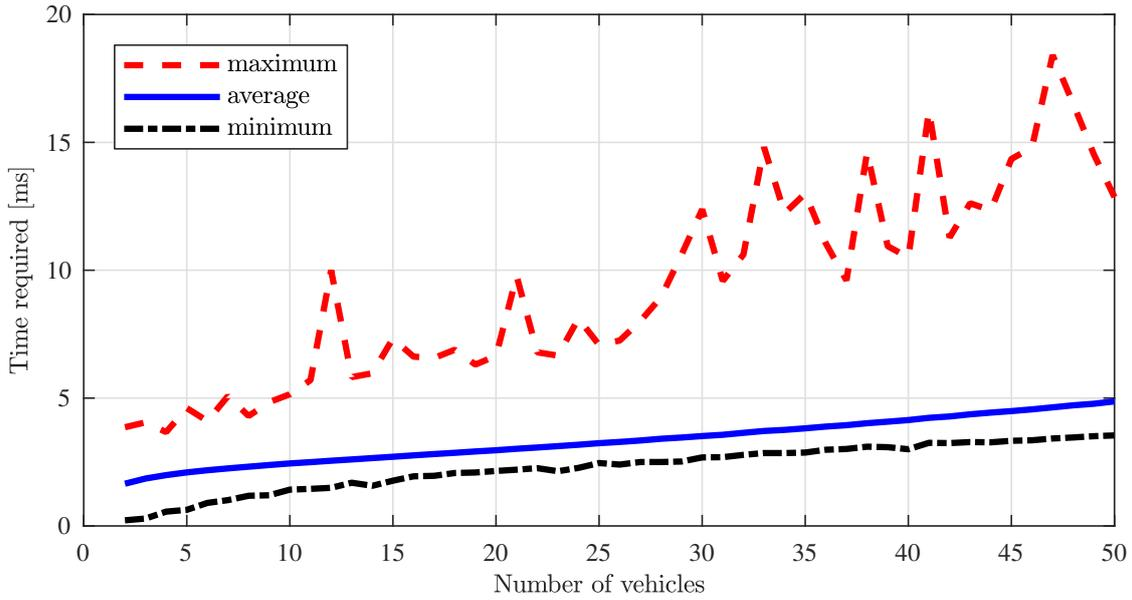
**Figure 5.8:** The required time for resolving the communication contention among the vehicles in RadCom using  $B_c = 40$  MHz, one-persistent CSMA with backoff value of 48.
