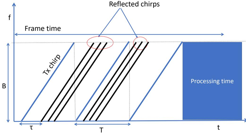
**Figure 3.1:** Frequency versus time FMCW chirp with reflected chirps from multiple targets.
