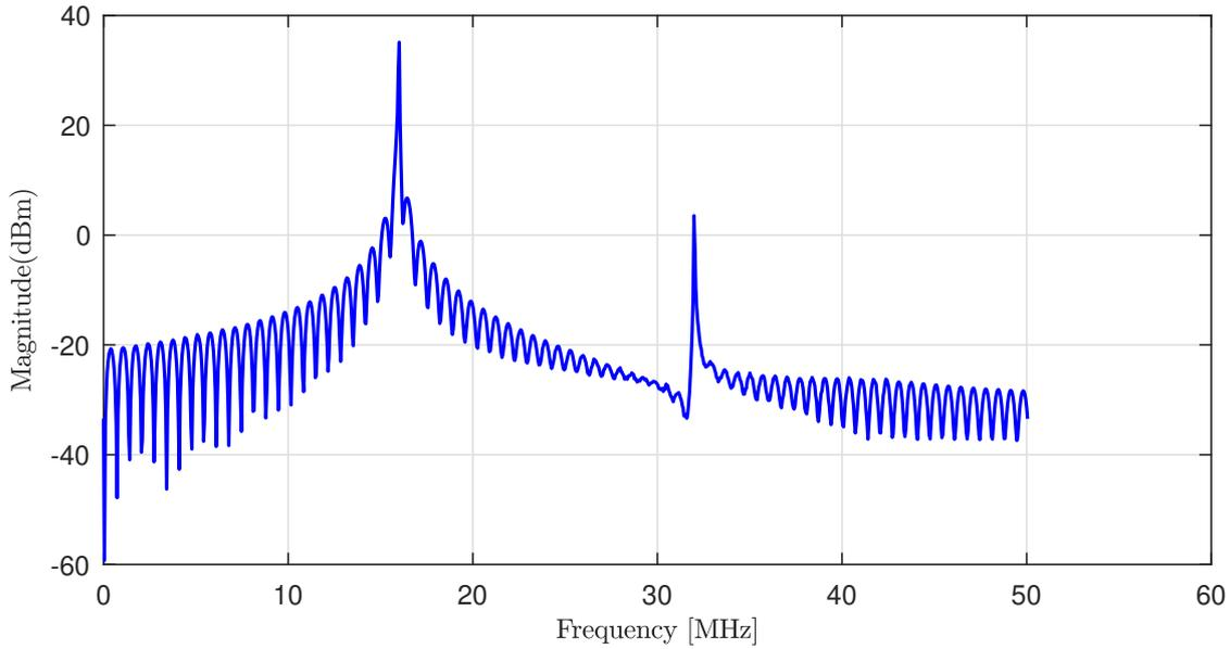
**Figure 3.4:** FFT of received signal containing interfering signal from a target located at a distance of  $d = 100m$ ,  $B = 1GHz$ ,  $T = 20\mu s$  and  $\tau = 0s$ .
