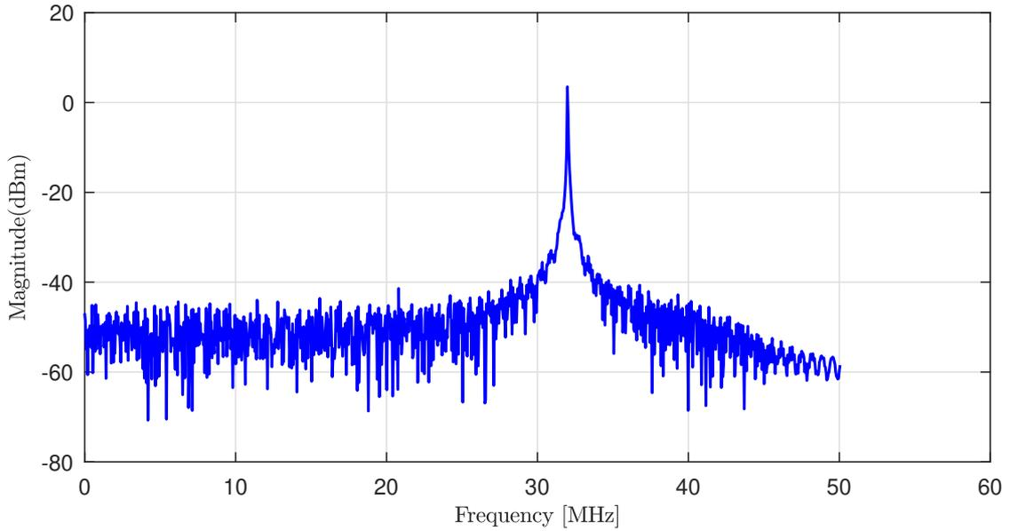
**Figure 3.3:** FFT of interference free received signal from a target located at a distance of  $d = 100m$ ,  $B = 1GHz$  and  $T = 20\mu s$ .
