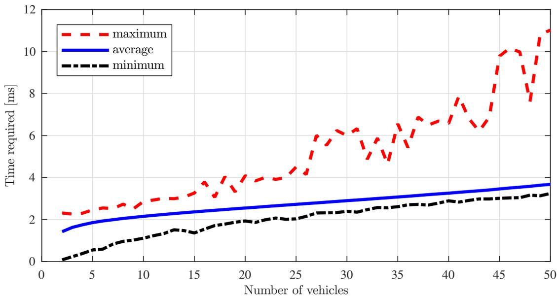
**Figure 5.7:** The required time for resolving the communication contention among the vehicles in RadCom using  $B_c = 40$  MHz, one-persistent CSMA with backoff value of 6.
