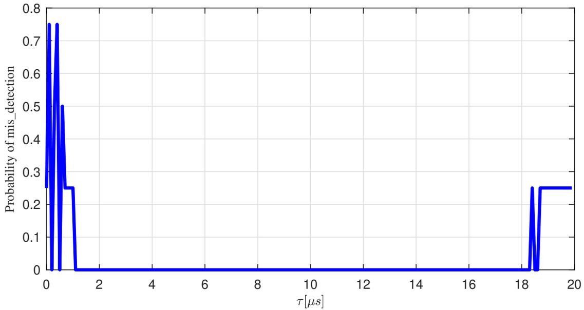
**Figure 5.3:** Probability mis-detection targets using radar only systems. The simulation contains four other interfering targets besides the ego target and the threshold value is  $7dB$ .
