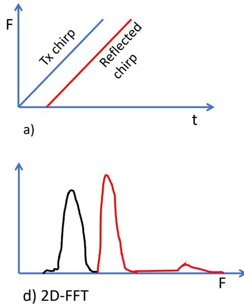
**Figure 2.11:** Resolving two objects located at the same distance but have different velocity using 2D-FFT.
