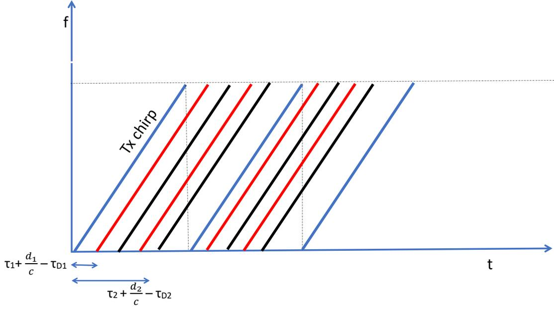
**Figure 3.2:** Reflected signals and mutual interference of signals from others around.
