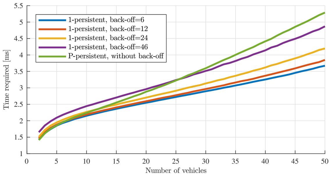
**Figure 5.10:** Comparison of time required for resolving the communication contention among the vehicles in RadCom using  $B_c = 40$  MHz between P-persistent CSMA without back-off and one-persistent CSMA with backoff.
