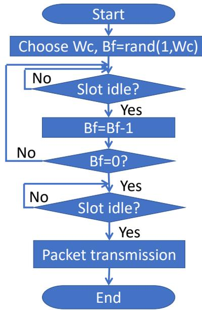
**Figure 4.2:** One-Persistent CSMA with backoff flowchart. Where  $B - f$  is backoff and  $W_c$  is the contention window.
