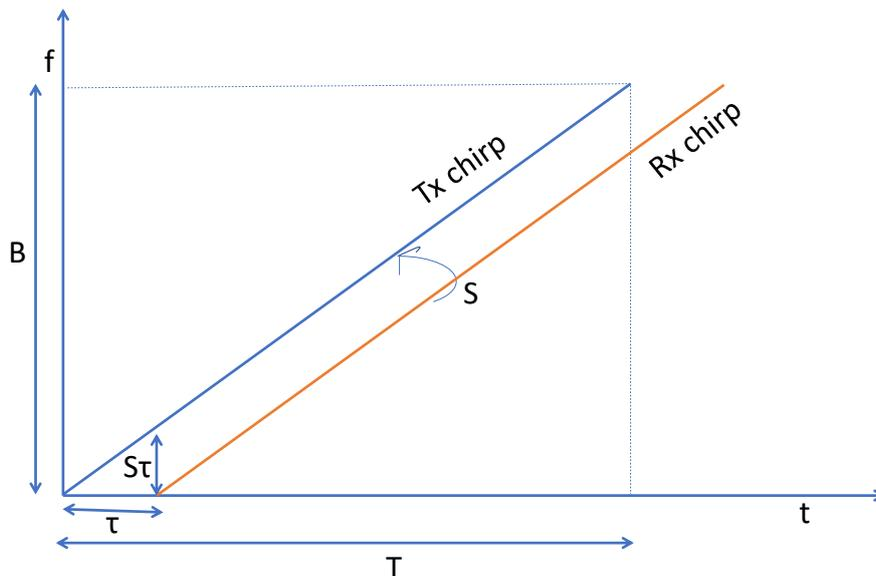
**Figure 2.2:** Sawtooth modulated chirp with frequency versus time plot.
