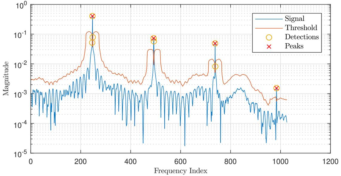
**Figure 5.5:** Target detection from output of the FFT signal using the implemented CFAR and the threshold value is  $10dB$ . We have more four interfering targets beside the ego vehicle.
