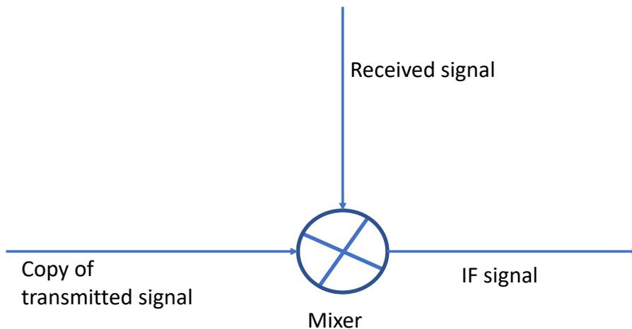
**Figure 2.4:** Copy of transmitted and signal and received signal feeding to mixer.
