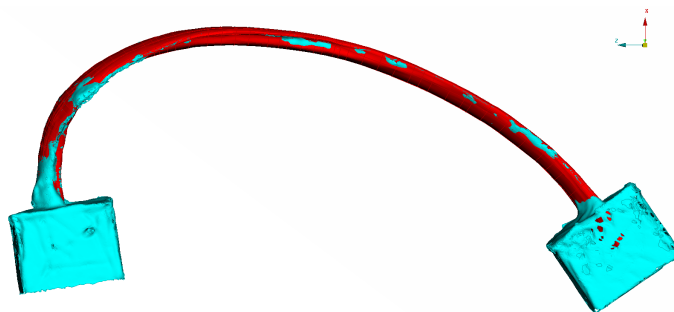
Figure 4.7: Hexahedral mesh (red) aligned with laser-scanned mesh (cyan).
