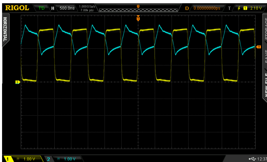
Figure 4.4: Oscilloscope image of the input and output voltage, when a 1 MHz square wave is applied to the system where C_{sol} = 1 nF and R_b = 560 \Omega .
