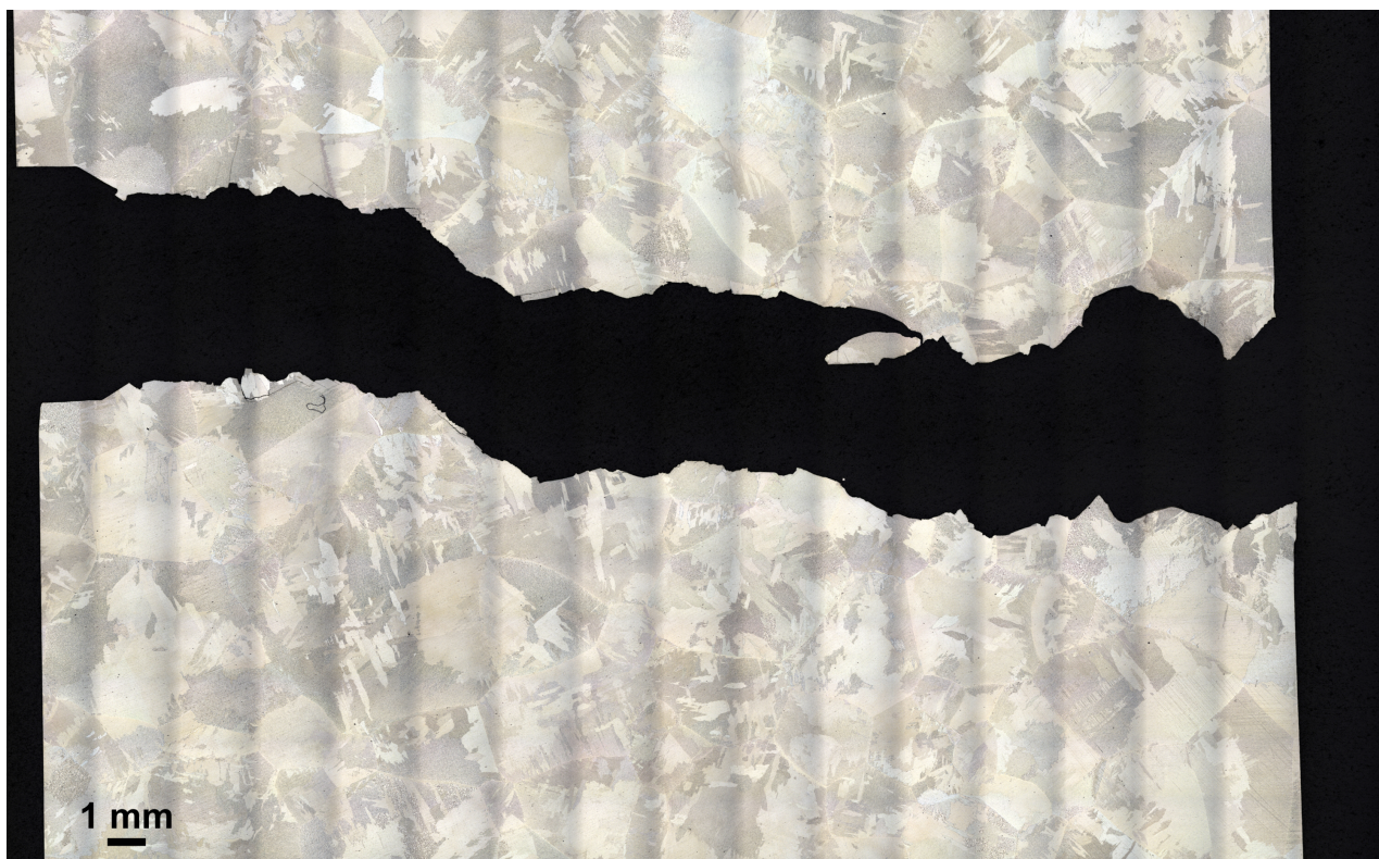
Figure B.1: Ti-64 grain size sample made from a C(T) specimen. The figure is composed by a number of pictures. The wave pattern is due to bad light conditions for each individual picture.
