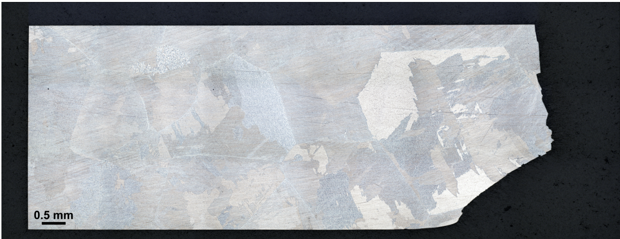
Figure B.3: Ti-64 grain size sample made from a Kb specimen. The figure is composed by a number of pictures.
