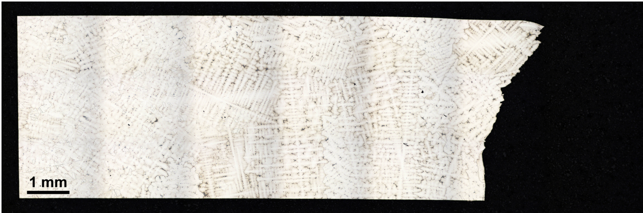
Figure B.5: IN-718 grain size sample made from a Kb specimen. The figure is composed by a number of pictures. The wave pattern is due to bad light conditions for each individual picture.
