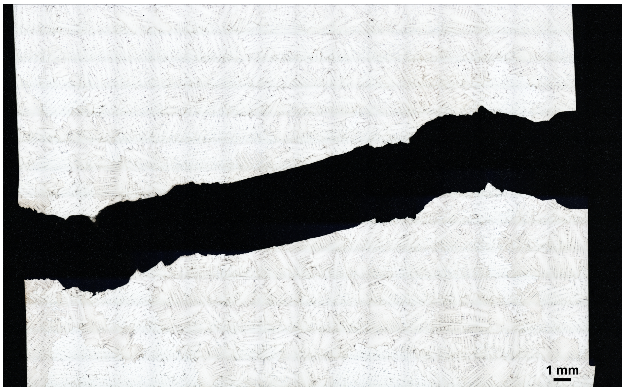
Figure B.4: IN-718 grain size sample made from a C(T) specimen. The figure is composed by a number of pictures. The wave pattern is due to bad light conditions for each individual picture.
