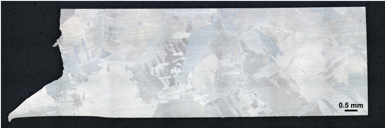
Figure B.2: Ti-64 grain size sample made from a Kb specimen. The figure is composed by a number of pictures.
