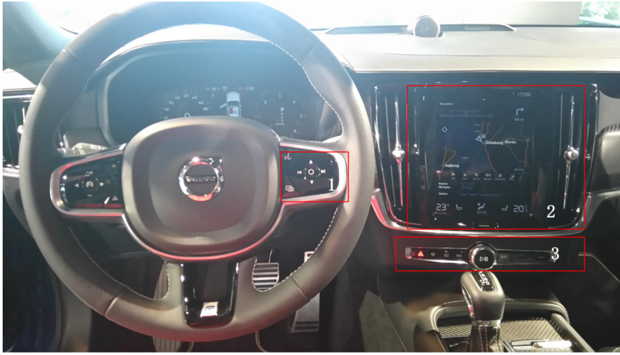
Figure 2.1: Infotainment system of Volvo S90, where 1. Voice control unit 2. Touch screen and 3. Keypads. Photograph taken by author.
