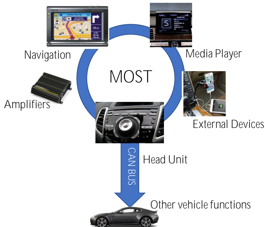
Figure 2.3: Infotainment system interaction architecture
