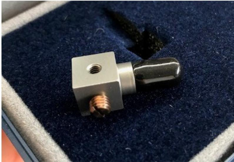
*Figure 3.1: The accelerometer SEN040F which are used during the measurements.*
