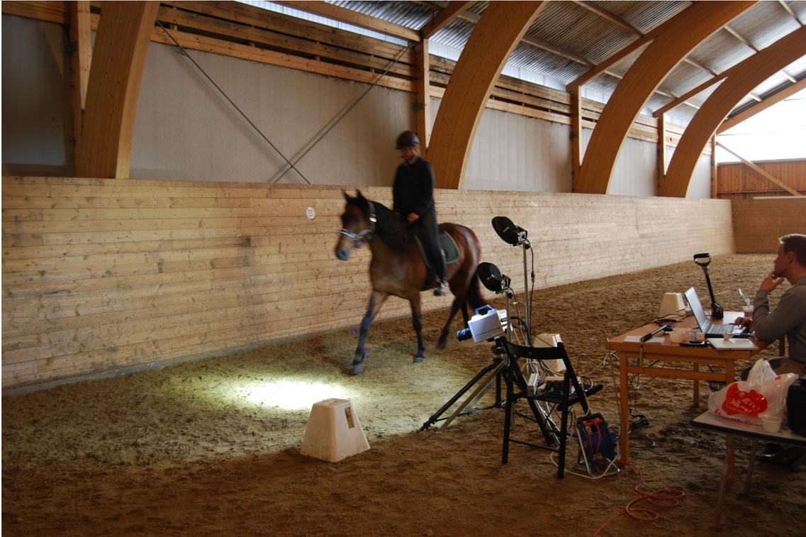
*Figure 4.5: The horse passes through the 10 m track where the measurements take place in the riding hall. Light beam visible on the ground from the high speed camera.*
