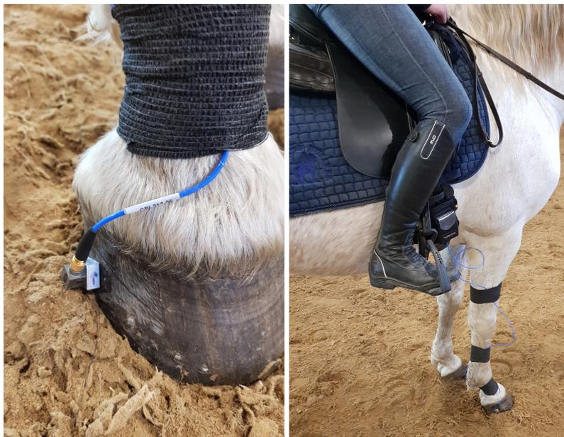
*Figure 4.4: How the accelerometer is screwed into the metal bracket and how the cord is fixed alongside the leg and into the logger.*
