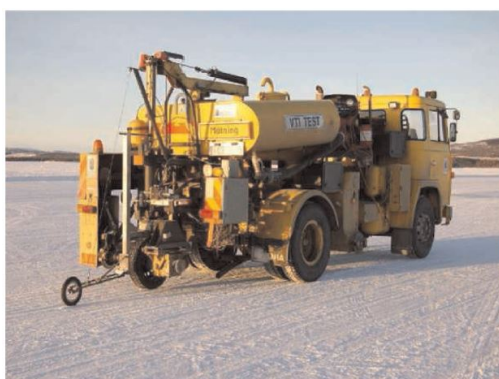
Figure 3.2: VTI's BV 12 Mobile Test Rig [15]
