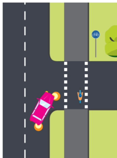
Figure 2.2 When a car has made a turn in an intersection and shall pass an unsupervised bicycle passage, the driver must drive at a low speed and give cyclists who are on or about to enter a bicycle passage an opportunity to cross (Transportstyrelsen, 2015a).
