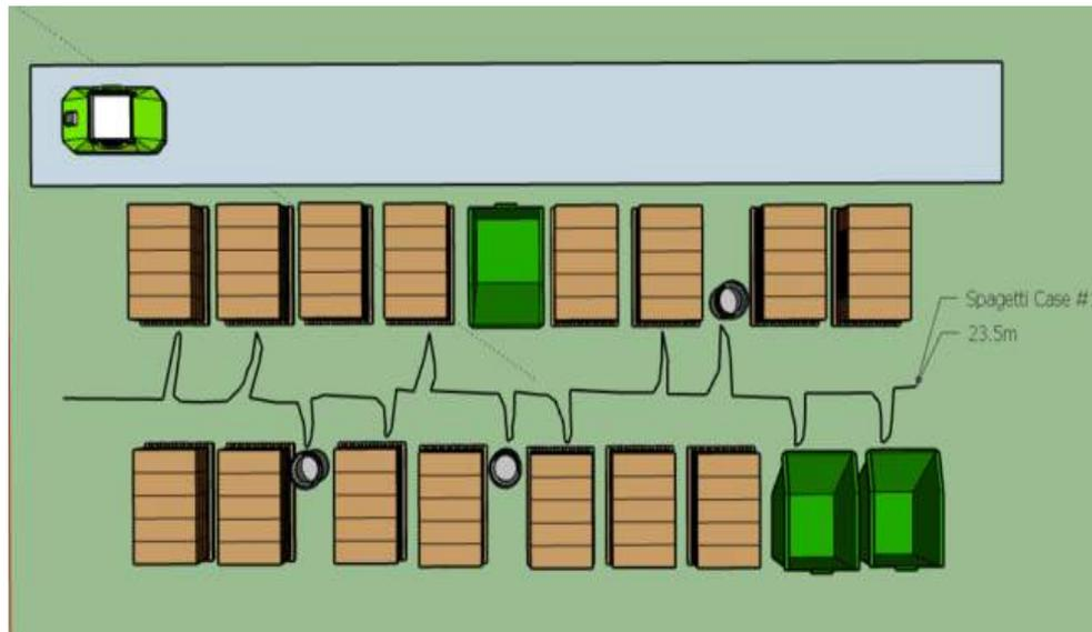
**Figure 1.10:** Spaghetti diagram of the operator path
