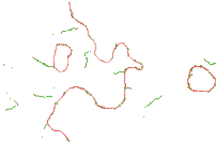
Figure 4.1: Result after letting the ants roam around for some time. Green patches represent the strength of scent trail, red agents are the ants.
