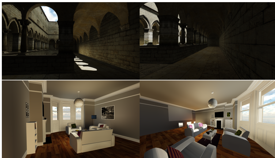
Figure 15: Direct and diffuse indirect light only, rendered using technique 1. Top row: SPONZA scene [9] with 8 \times 8 \times 4 = 256 probes. Bottom row: LIVING ROOM scene [9] with 3 \times 3 \times 4 = 36 probes.
