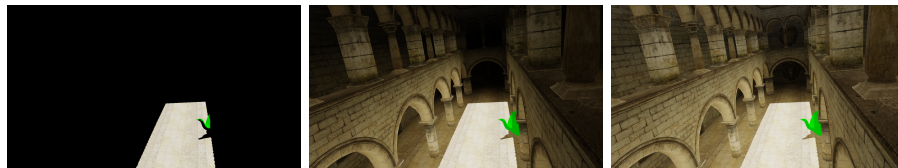
Figure 19: From left to right: SPONZA rendered without indirect light, 8 propagation iterations, 16 propagation iterations. All without ambient light. Many dark spots that should be lit are still visible when using 8 propagation iterations.
