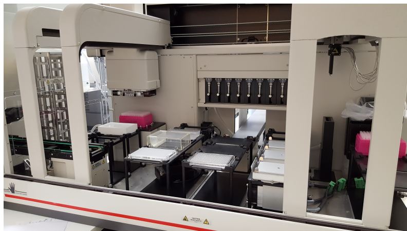
Figure 3.6: The Biomek FX P laboratory automation workstation was used to pipette qPCR master and transfer diluted cDNA in the 384-well plate.
