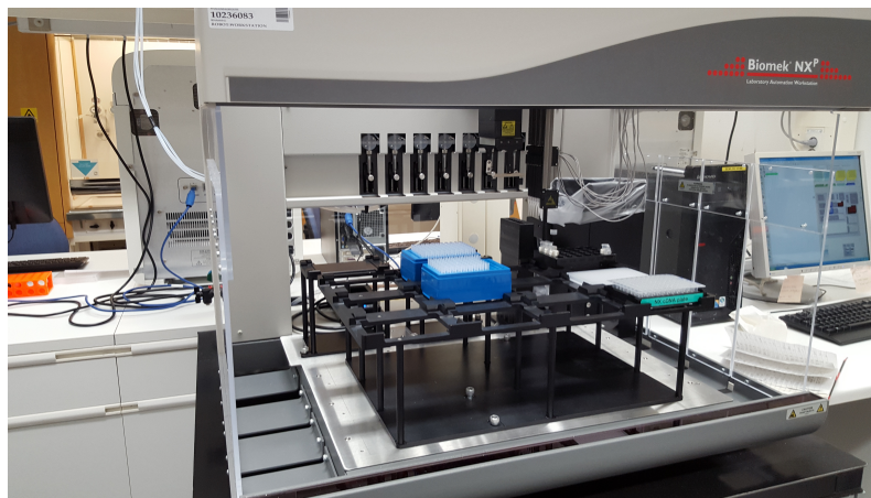
Figure 3.5: Biomek NXP liquid handler used for pipetting qPCR master mix and transferring cDNA template from a 96-well plate.
