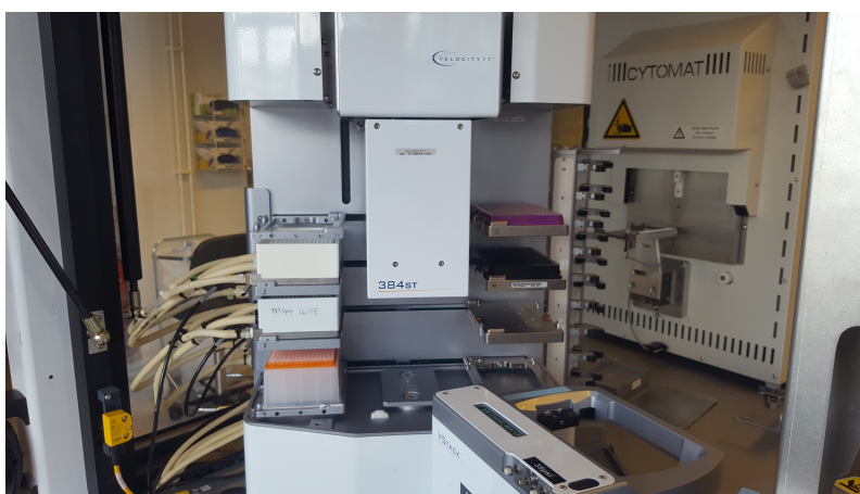
Figure 3.4: VPrep Liquid Handling Pipetting Station that was used for transfer of lysate to the rigid 384-well PCR plate containing RT master mix.
