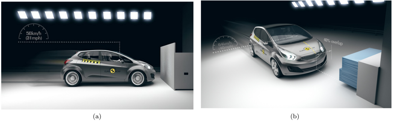
Figure 6.9: Setup for the FWRB crash test in 6.9a and ODB in 6.9b [34]
