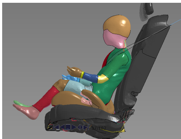
Figure 8.16: Rotational kinematics derived from interaction between the belt guides and the belt configuration.
