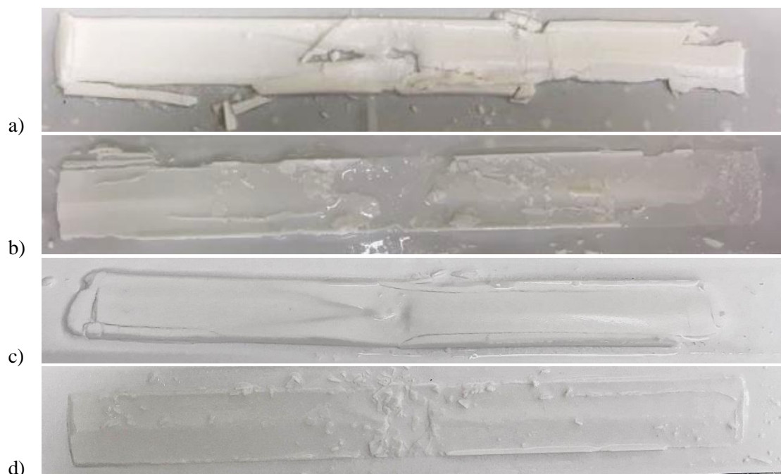
Figure 12. Photos of the membranes and fouling layers after FDG measurements. a) pH 2.9, regenerated cellulose membrane, b) unadjusted pH, regenerated cellulose membrane, c) pH 2.9, polyethersulfone membrane, d) unadjusted pH, polyethersulfone membrane
