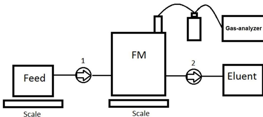
**Figure 3.1:** Schematic overview of the chemostat set-up, 1 & 2 are showing pumps and there is further a safety bottle between fermentor (FM) and off-gas analysis.
