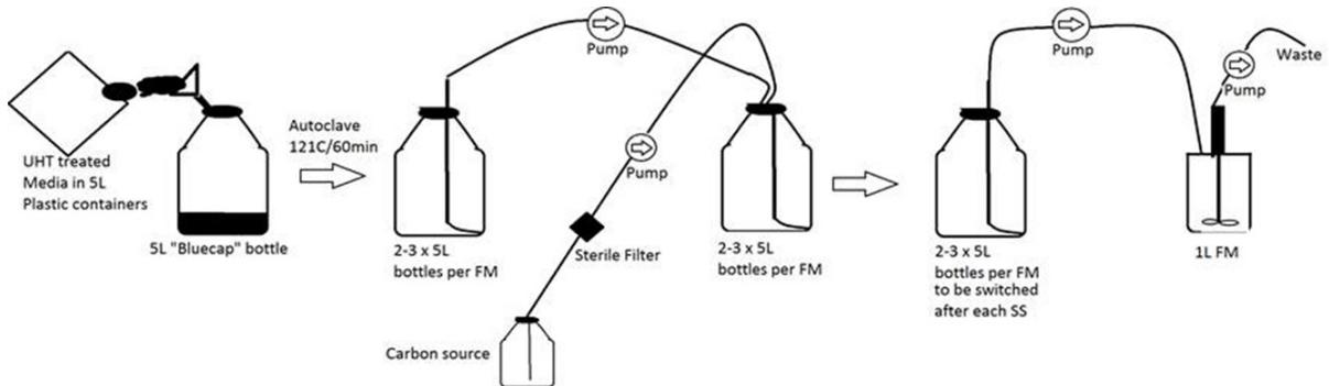
**Figure 3.2:** Schematic overview of the medium preparation set-up.
