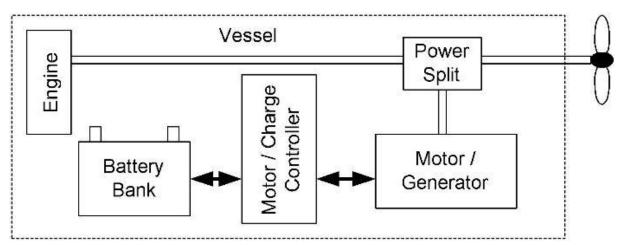
Figure 7 basic overview of a parallel hybrid. (Hybrid-Marine LTD, 2008) Reprinted with permission.
