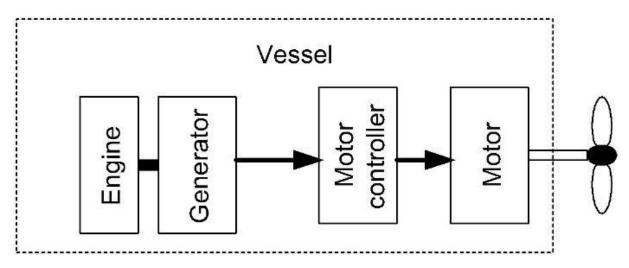
Figure 5 basic overview of a diesel/electric system and how it fits together. (Hybrid-Marine LTD, 2008) Reprinted with permission.
