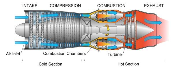
Figure 1 a cross section of a gas turbine to show how it works from the compression to the exhaust. (Wikipedia, reprinted with permission).
