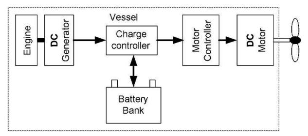
Figure 6 basic overview of a serial hybrid. (Hybrid-Marine LTD, 2008) Reprinted with permission.
