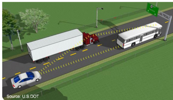
Figure 2.6: A demonstration of the V2V communication (sidelink) through the PC5 interface
