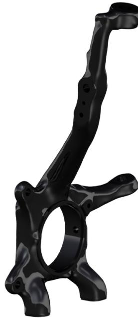
**Figure 3.20:** 3D scanned OEM upright
