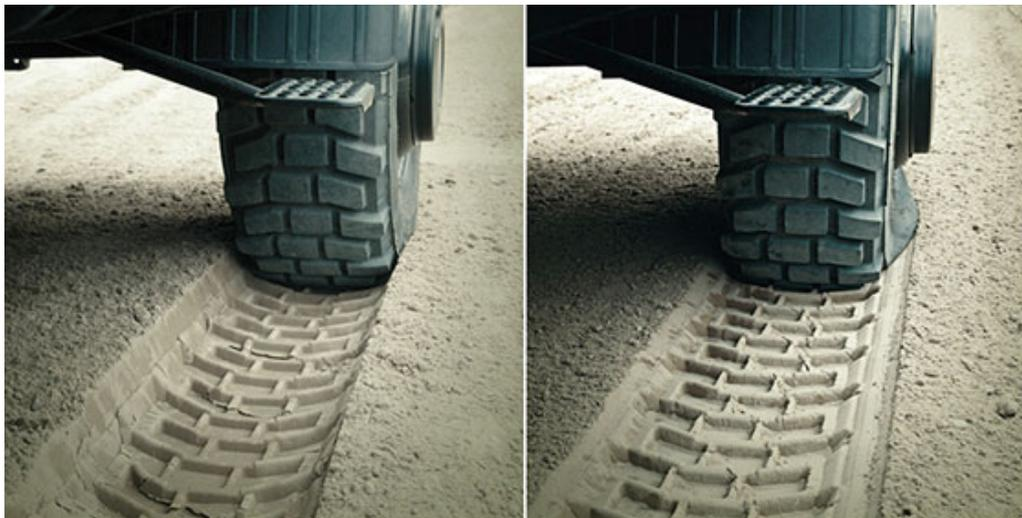
**Figure 3.30:** CTIS in action on Unimog [44]
