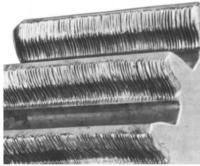
**Figure 2.9:** Typical example of Abrasive wear. [46]
