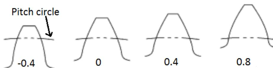
**Figure 2.11:** The affect of profile shift on gear tooth for 30 teeth gear wheel. [10]
