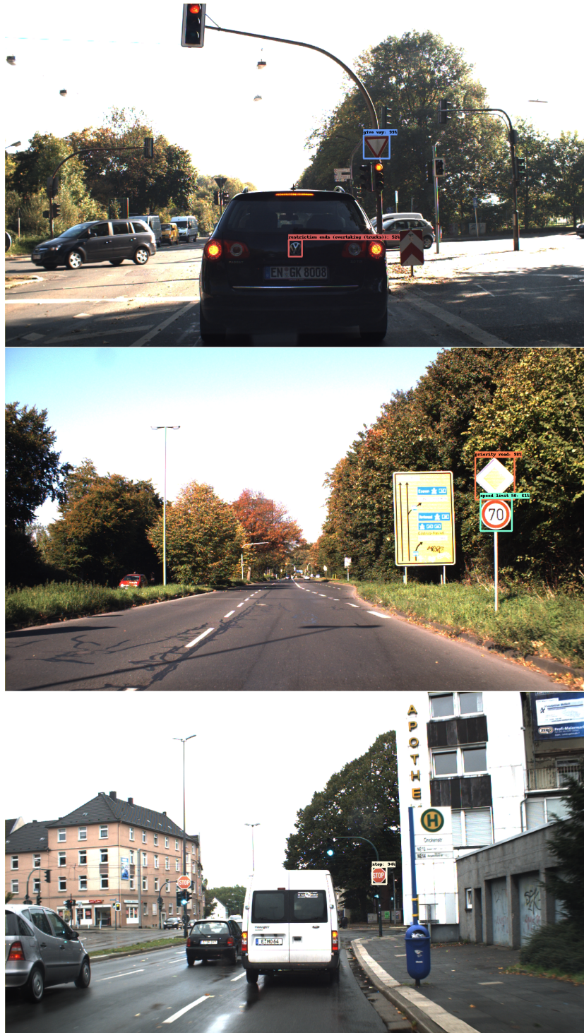
Figure 4.23: Example output from the test set after training the Faster R-CNN model on the extended training set. In the top image the model incorrectly predicts the Volkswagen-logo as a sign. In the middle image the Priority road sign is correct, but the network classifies the 70-sign as a 50-sign. In the bottom image the network fails to find and classify the left stop sign.
