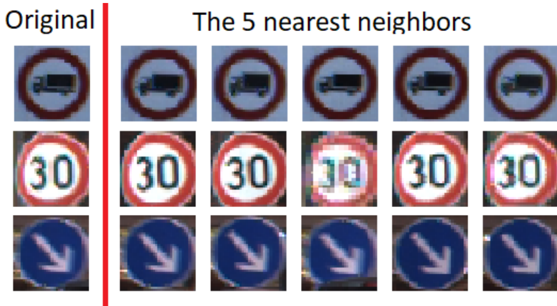
Figure 5.2: The 5 nearest neighbors of three randomly chosen images in the GT-SRB test set, calculated in L1-norm. All other observed images gave equivalent results, as well as when calculating nearest neighbors in L2-norm. It is evident that many images in the test set are very alike, suggesting that the intraclass homogeneity is high - which is what to expect since traffic signs of a specific class are specifically created to resemble each other perfectly.
