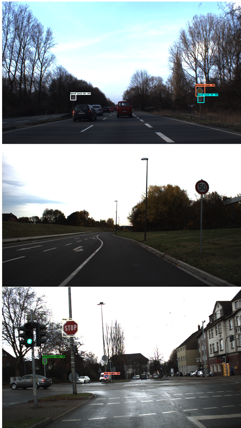
Figure 4.22: Example output from the test set after training the Faster R-CNN model for 150000 steps on the original training set. In the top image it can be seen that the network makes a correct prediction of the Priority road sign and it does find both 70-signs. However the speed signs are wrongly classified as 60 and 30. In the middle picture the network does not find the 50-sign. In the bottom picture the stop-sign and keep right-sign are both predicted correctly, however in the left part of the picture the presence of a sign is wrongly predicted.
