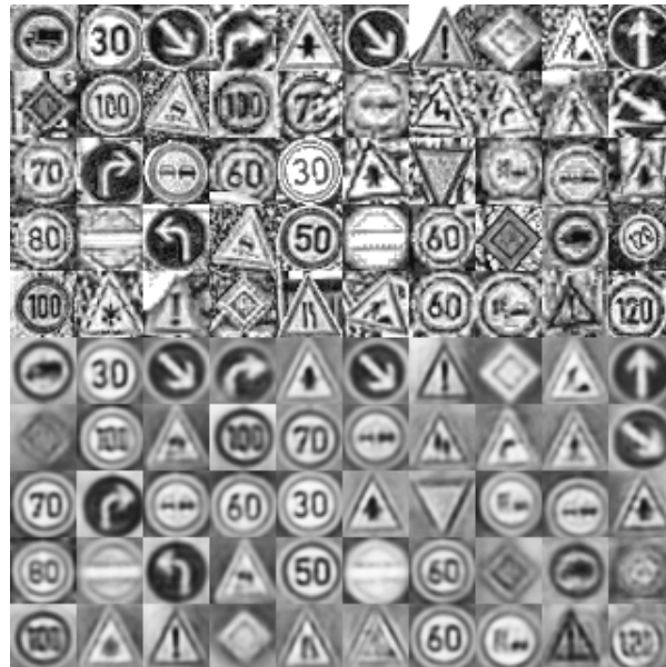
Figure 4.18: Input traffic signs and the corresponding reconstructed images by the decoder network. The real are on the upper half of the image and the reconstructed on the lower half.
