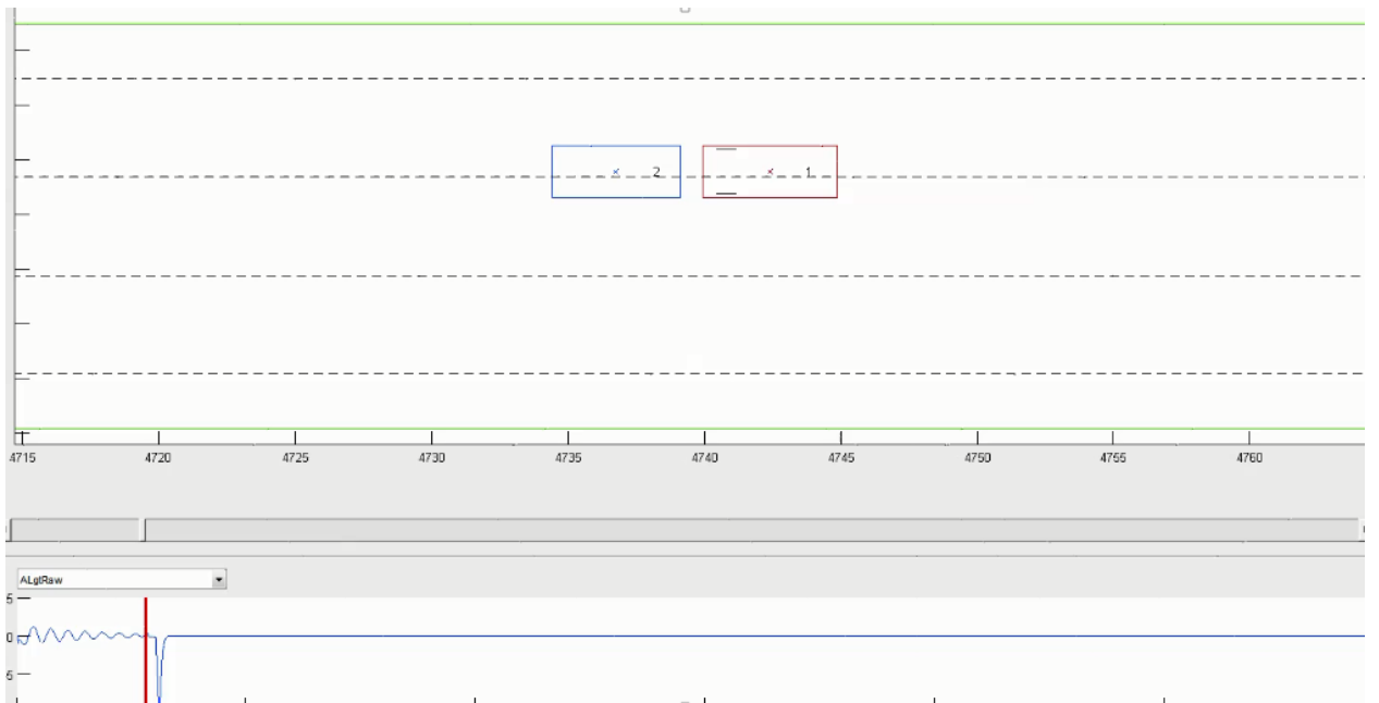
Figure 6.4: CLR test. In this figure one of the critical situation is found on the map, the curve right beneath the BirdView is the reaction of deceleration. The AD car is braking with the help of ASFG, there is deceleration on the host vehicle but it does not fully stop the car before the collision happens. This means the braking function, while working great under perfect CCR tests, is not performing as good in close-to-real-life scenarios. This is to be reported to the engineers developing ASFG and further tests will be done in the future to improve the braking function.
