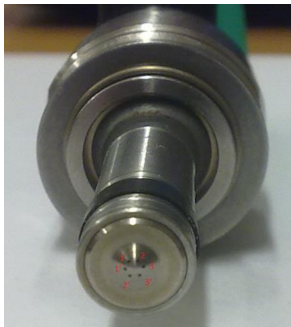
Figure 12: Six hole multihole injector, nozzle tip
