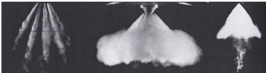
Figure 24: Spray formation from three different types of injector, multihole, outwards opening, swirl type (Skogsberg, 2007)
