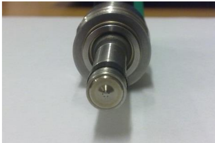
Figure 4: Injector, hole configuration
