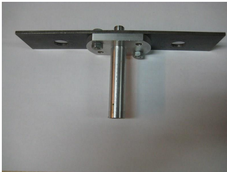
Figure 11: Upper injector mounting
