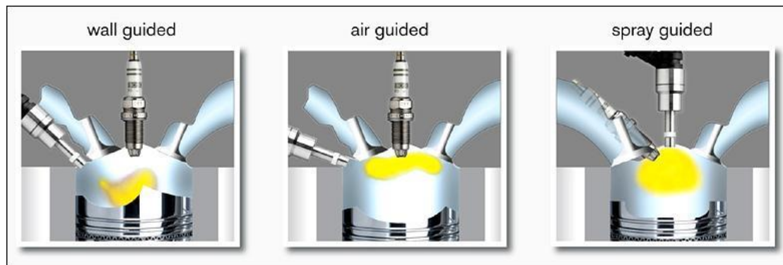
Figure 23: Comparison of three different injection systems (Xander, 2006)
