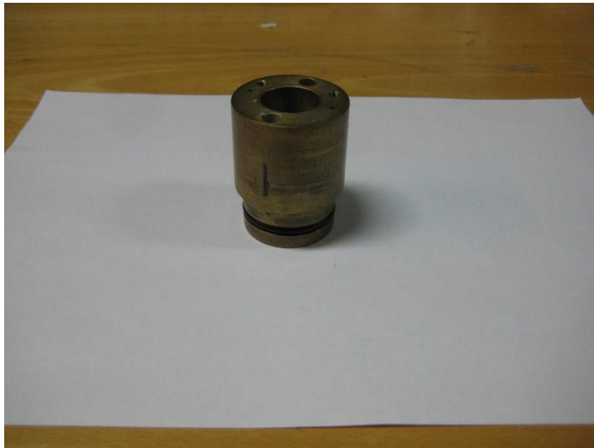
Figure 9: Lower injector mounting
