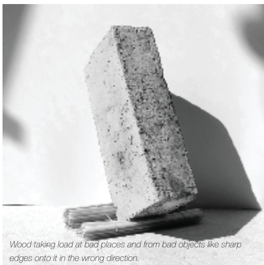
Wood taking load at bad places and from bad objects like sharp edges onto it in the wrong direction.
